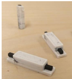
Figure 5. Horizontal and vertical dual extrusion samples.
