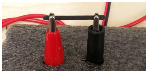
Figure 3. A horizontal block sample being tested for resistivity
