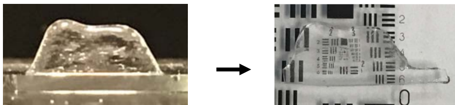
Fig. 7. 2D wall post-deposition (left), after polishing to create transmissivity sample (right)
