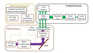
Fig. 1. The integrated ECPL system: ECPL process, ICM&M module, and MATLAB software for ECPL M&C
