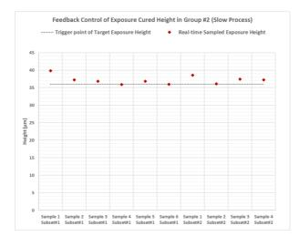
Fig. 6. Real-time feedback control results for exposure height in the real-time measurement and control experiments Group #2
