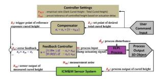
Fig. 3. Scheme diagram of feedback control for real-time cured height in ECPL process
