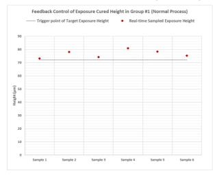
Fig. 5. Real-time feedback control results for exposure height in the real-time measurement and control experiments Group #1
