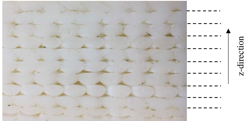
Figure 1. Cross section of an extrusion-based 3D printed part showing layered architecture.
