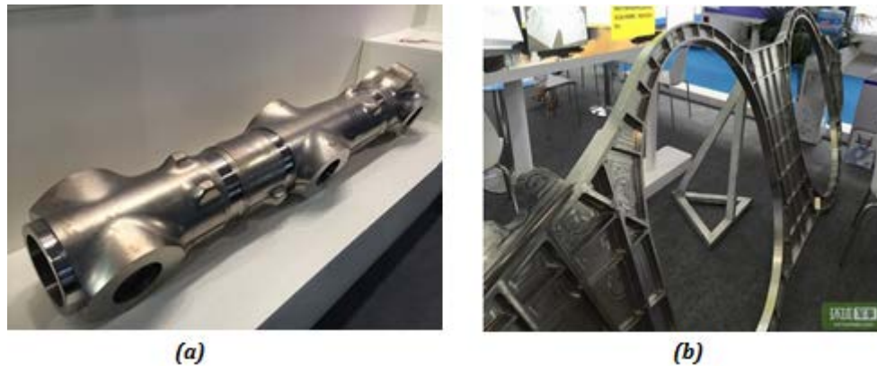
Fig. 2. Sample aircraft parts made of Titanium. (a) Forged landing gear [6] (b) 5m 2 3D-printed Titanium alloy load-bearing frame [7]
