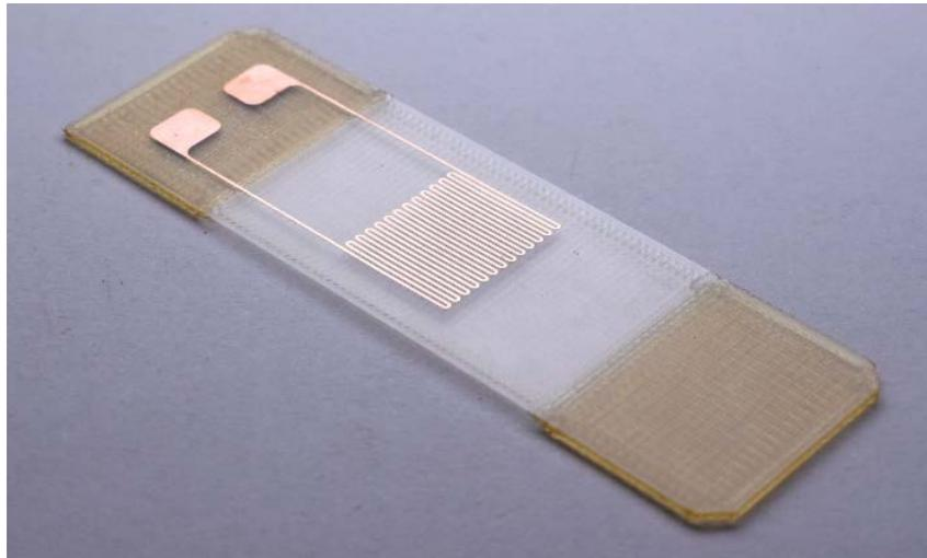
Figure 5: Plated sensor with a 10 mm grid consisting of 32 elements at a 500  $\mu\text{m}$  pitch.
