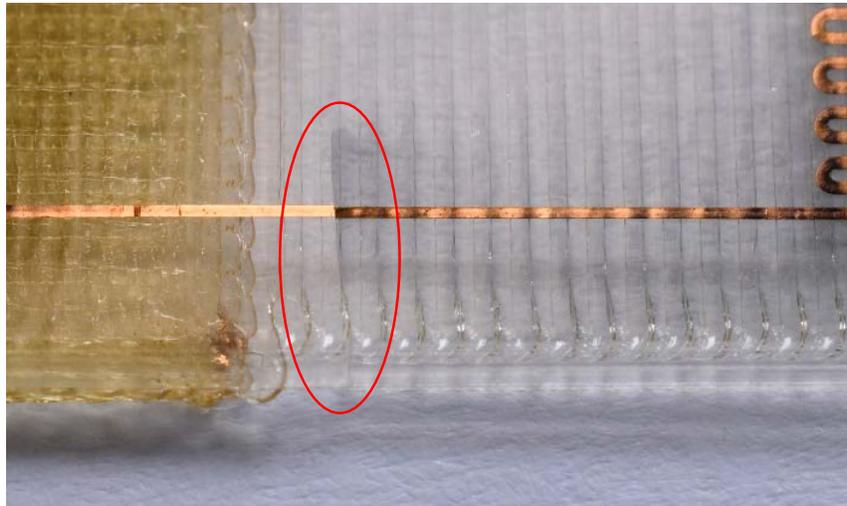
Figure 9: Close-up image of the failure point of the sensor. Note the crack running parallel to the infill direction through both substrate and copper (highlighted in red).
