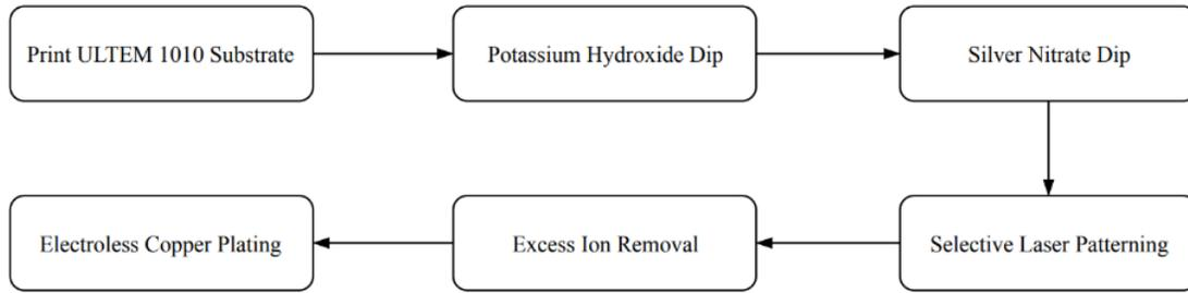
Figure 2: Generalized process flowchart for manufacturing ULTEM 1010 based electronics
