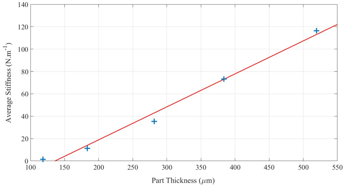
Figure 7: Graph showing average stiffness (K) vs substrates thickness.
