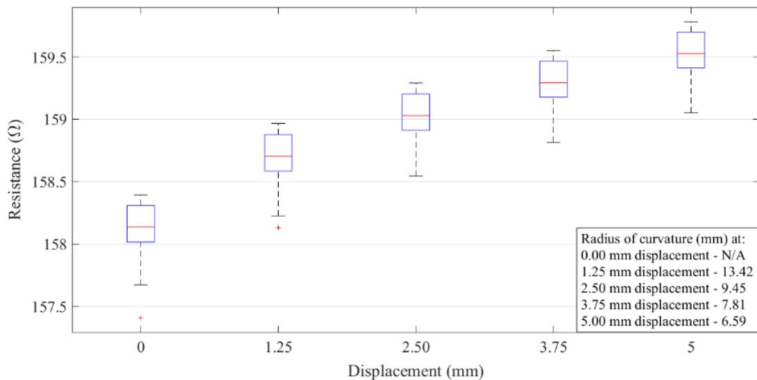
Figure 11: Boxplot comparing change resistance with linear compression over 4000 cycles.
