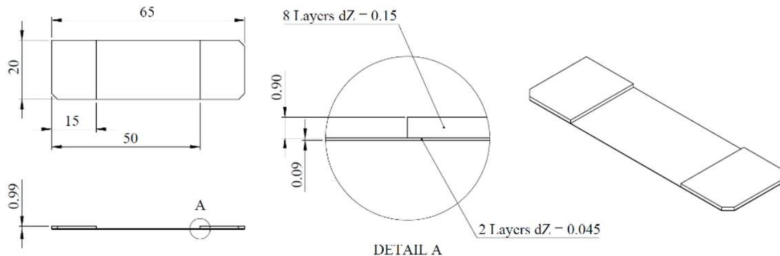
Figure 3: Schematic layout of positional sensor substrate
