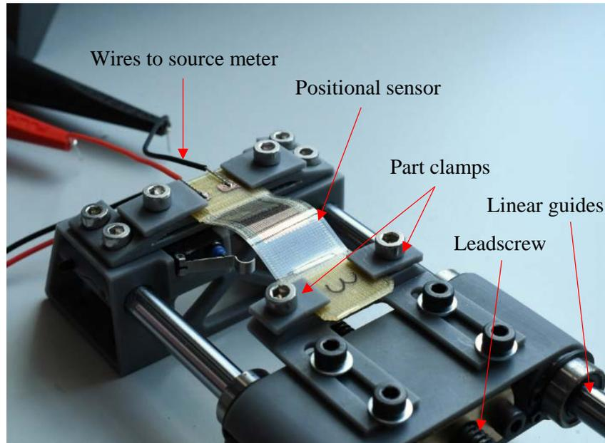
Figure 6: Positional sensor undergoing cyclic testing in the linear compression rig.
