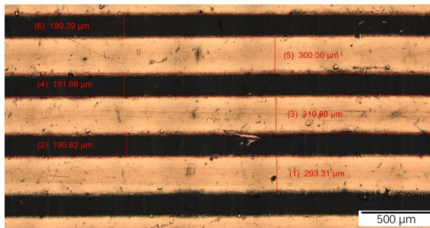
Figure 4: Optical microscope image of positional sensor grid illustrating track and gap sizes.
