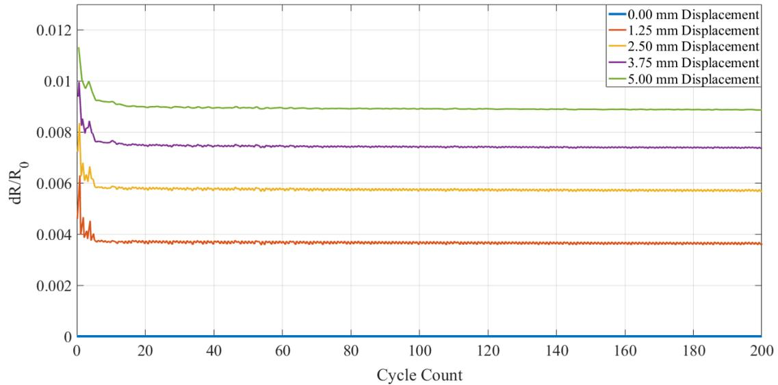
Figure 10: Graph showing variation of percentage change in resistance after 200 cycles at different compressions.
