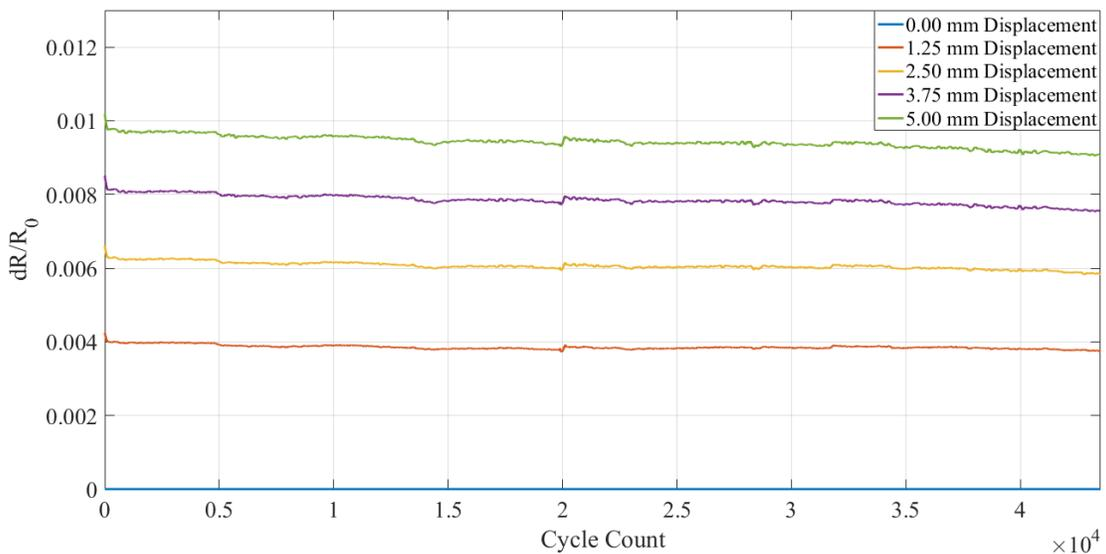
Figure 8: Graph showing variation of  $dR/R_0$  over the lifetime of a sensor.
