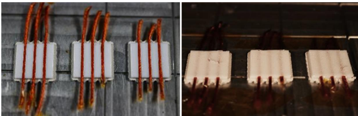
Figure 8: Embedding of kapton coated litz wire in circular cavities
