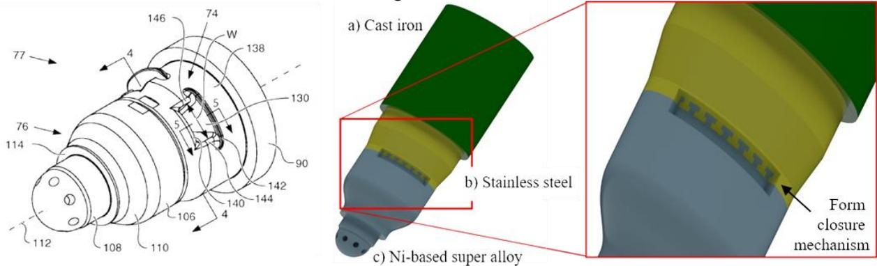
Figure 2: Pre-chamber of internal combustion engine. Left side: Excerpt from patent [7]. Middle and right side: Replica of the multi-material part with visualized material zones. The zoomed view of the right picture shows a possible interlocking between the two material zones to ensure a mechanical force transmission.
