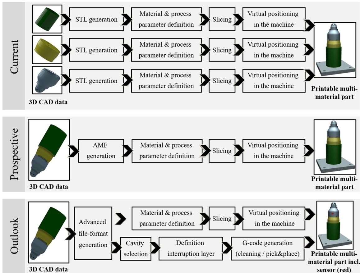
Figure 3: Data flowcharts for the production of mechatronic multi-material parts: current, prospective and outlook.
