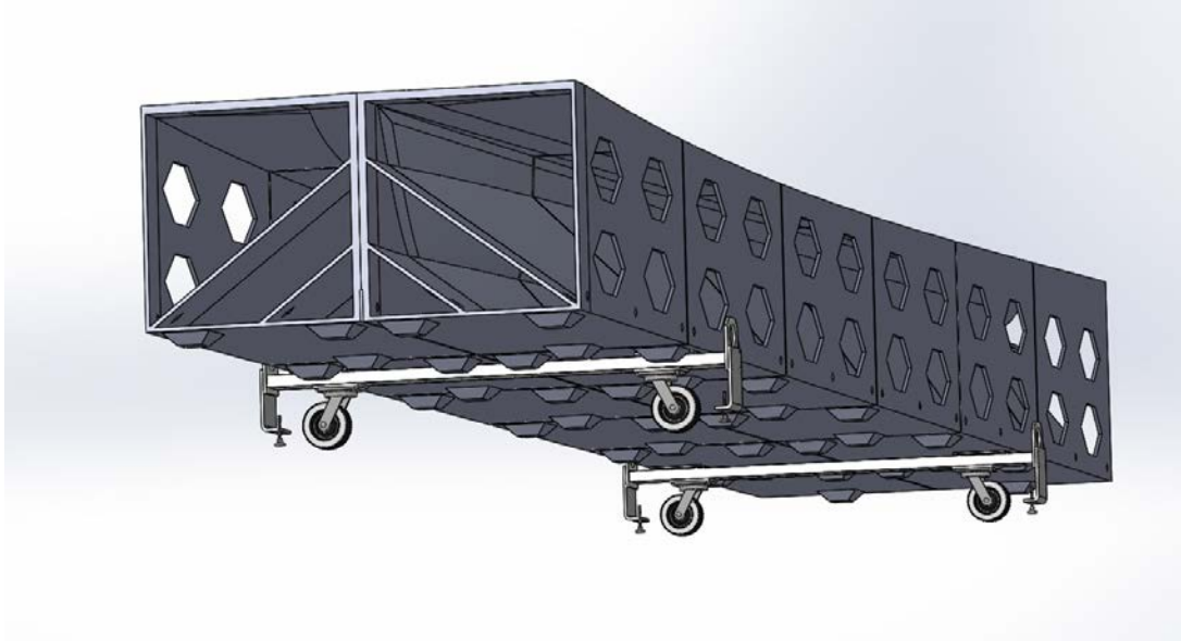
Figure 7: Caster arrangement on boat hull mold.
