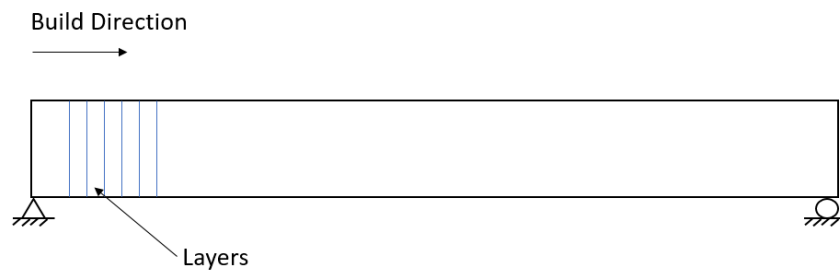
Figure 3: Illustration of the build direction going down the length of the part.
