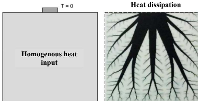
Figure 1: TO for optimal heat transfer at the center of the top edge of a heat generating solid [5]
