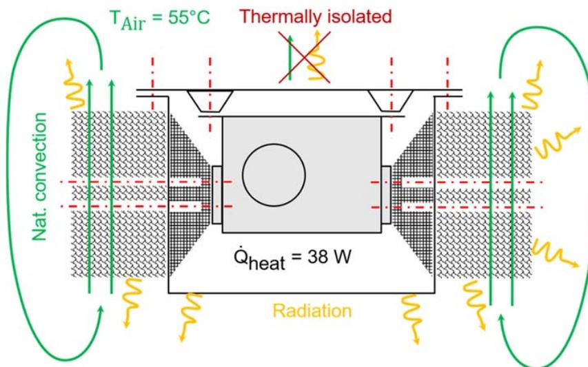
Figure 4: Schematic sketch and operating principle of the housing
