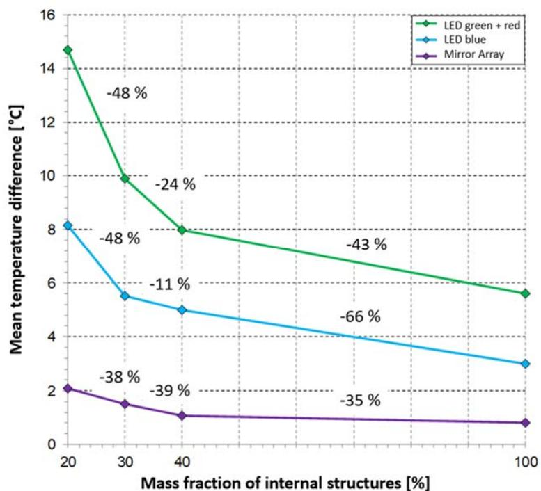
Figure 8: Mean temperature difference in correlation to mass fraction of internal structures
