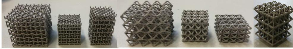
Fig.3 Some fabricated Ti6Al4V samples
