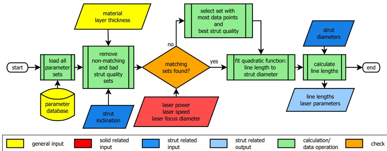
Figure 4: Flowchart of line length estimation for Pseudo-P-exposure
