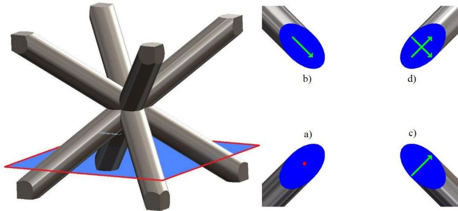
Figure 3: Slicing of a single BCC unit cell – left: slicing plane
