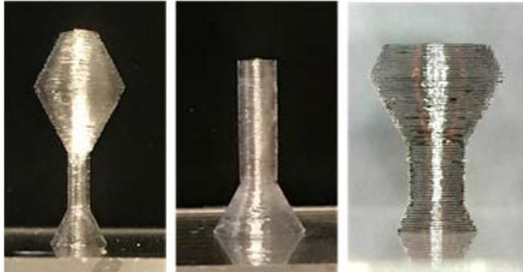
Fig. 5. Simple geometries deposited with quartz SMF
