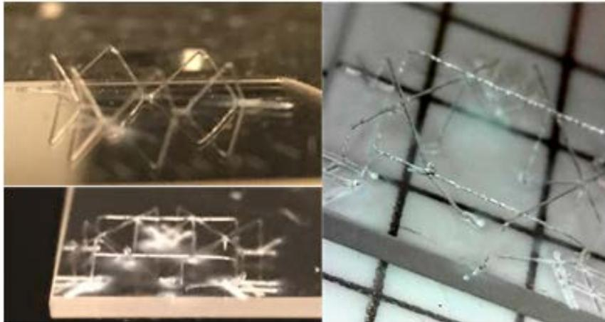
Fig. 7. Fiber truss in various stages of deposition
