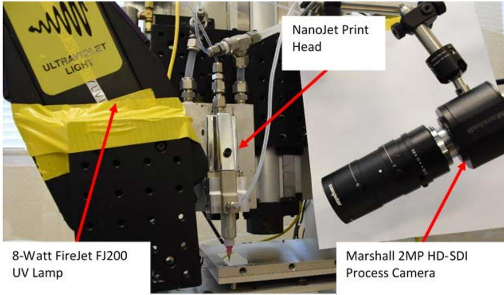
**Figure 1.** Photograph of the NanoJet system used in this study. The system features a Marshall compact 2MP HD-SDI camera for process monitoring, an 8-Watt FireJet FJ200 UV lamp for soft curing of the material, and the printhead to house, aerosolize, and deposit the materials of interest.
