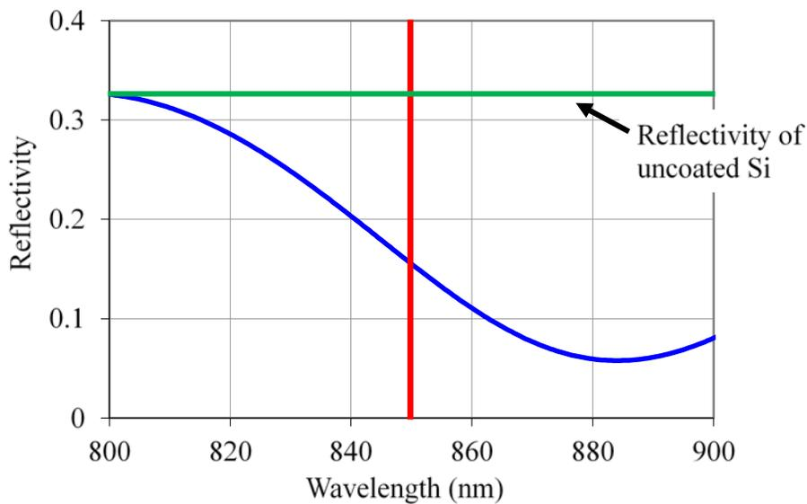
**Figure 11.** Reflectivity of the film printed with the 20:1 ink for wavelengths from 800-900 nm. The green line represents the typical reflectivity of the uncoated Si substrate, which was approximately 33%. The red line represents the emphasized wavelength of 850 nm, at which the film had a reflectivity of approximately 17%.
