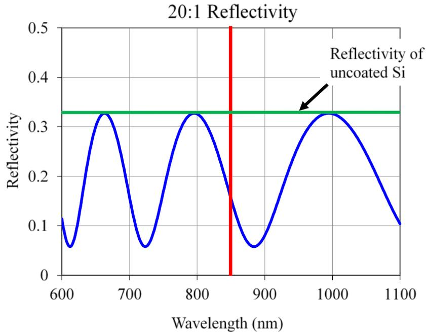
**Figure 10.** Reflectivity of the film produced with the 20:1 ink from 600-1100 nm. The green line represents the typical reflectivity of the uncoated Si substrate, which was approximately 33%. The red line represents the emphasized wavelength of 850 nm, at which the film had a reflectivity of approximately 17%.
