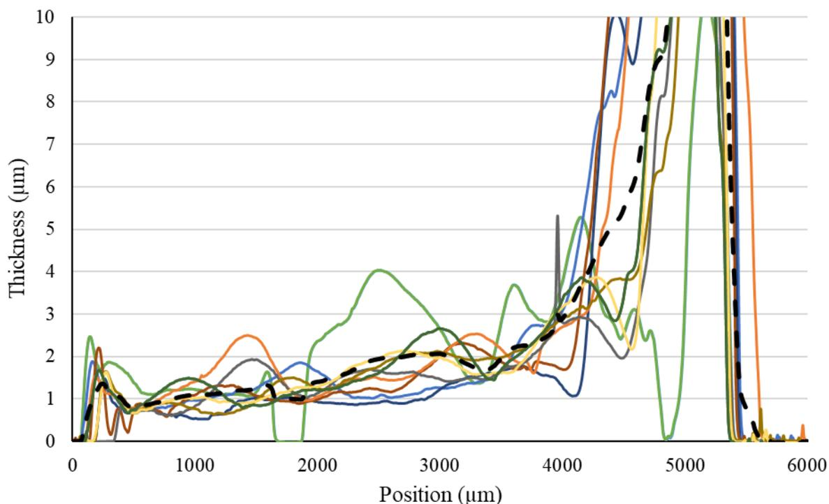
**Figure 9.** Plot of 11 measurements of thickness of a single film produced with the 20:1 material, as well as the average of the data sets. The Y-axis has been adjusted to offer a better view of the data.
