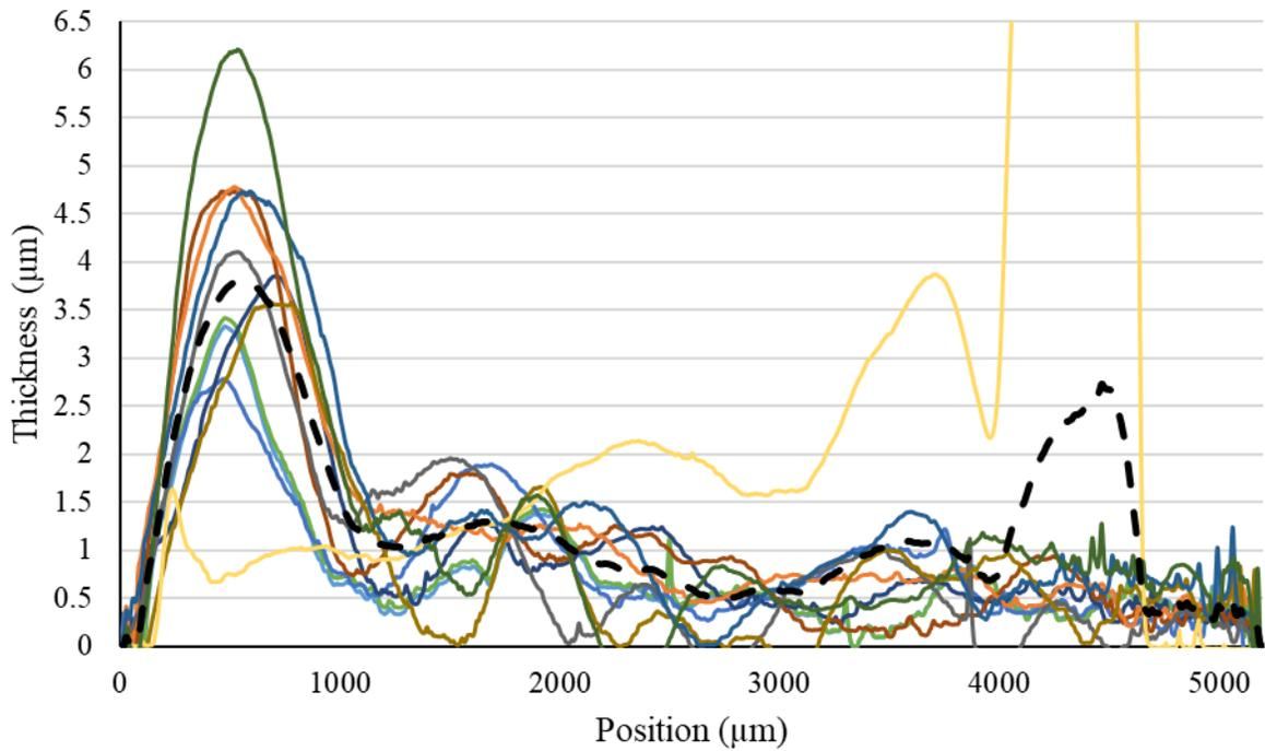
**Figure 7.** Plot of 11 measurements of thickness of a single film produced with the 14:1 material, as well as the average of the data sets. The Y-axis has been adjusted to offer a better view of the data.
