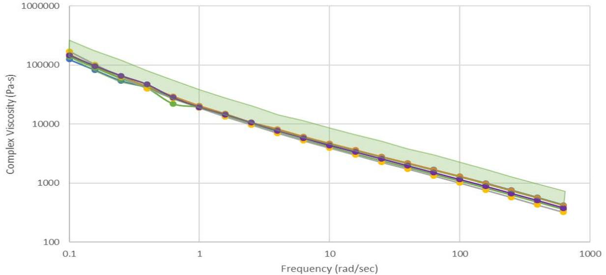
Figure 8. Graph of viscosity data of five presheared samples, overlaid with the range of viscosity of normal samples (20% CF ABS, 250°C, Air, 0.1% strain)
