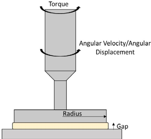
Figure 1. Model of parallel plate rheometer
