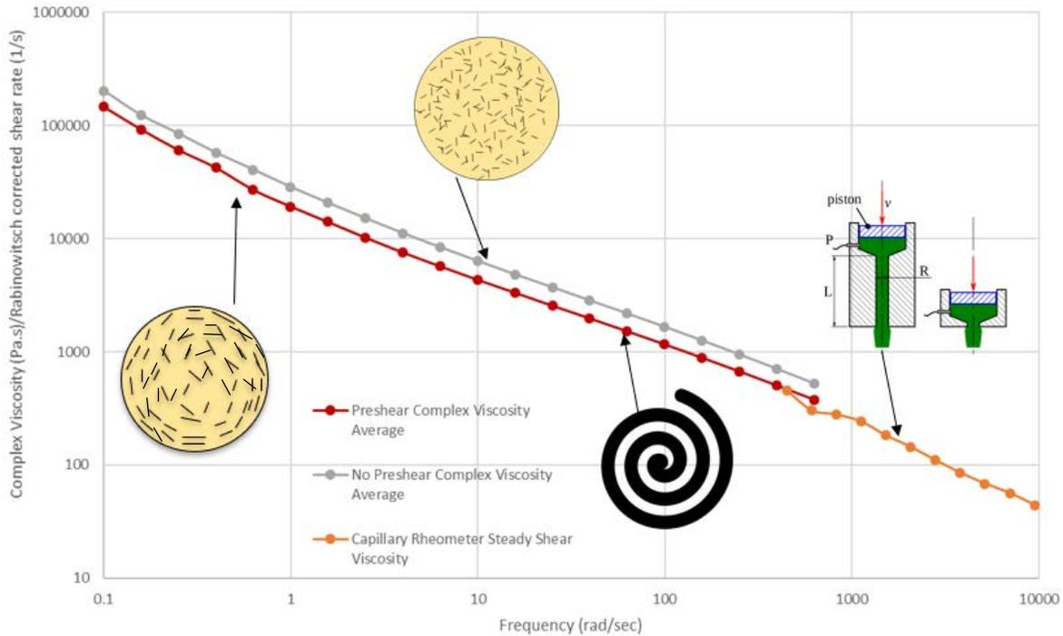
Figure 9. Graph comparing averaged viscosity data to viscosity data from a capillary rheometer and a printed specimen (20% CF ABS, 250°C, Air, 0.1% strain)
