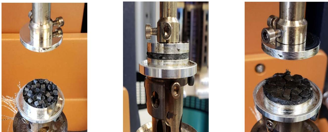
Figure 4. (from left to right) Pellets loaded in melt ring, pellets after melting, before testing, different view of pellets after melting, before testing
