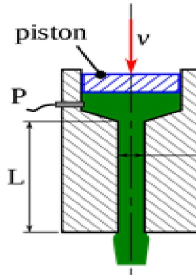
Figure 2. Model of capillary rheometer
