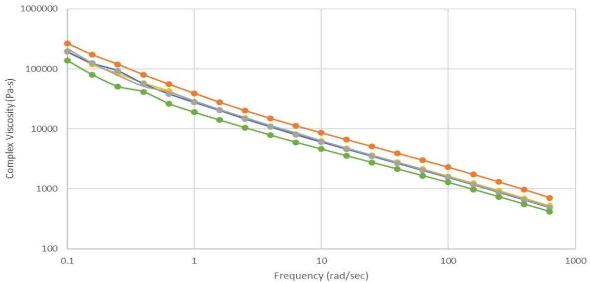
Figure 6. Scatter seen in viscosity data of randomly loaded samples (20% CF ABS, 250°C, Air, 0.1% strain)
