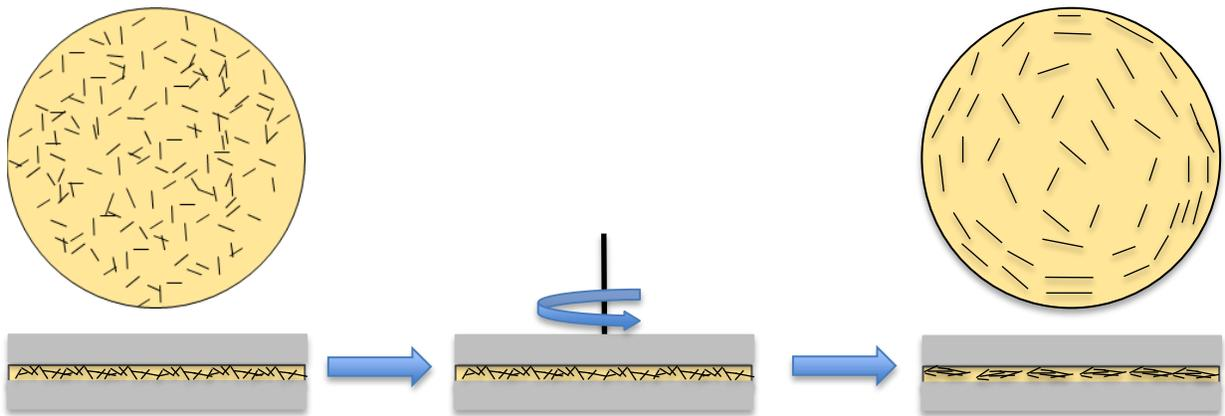
Figure 5. (from left to right) Model of both plates with melted random sample, model depicting the rotation of the upper plate to shear the sample, hypothesized model where fibers are given some alignment from the pre-shearing process
