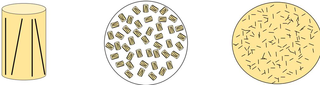
Figure 3. (from left to right) model of carbon fiber reinforced pellet, top-down view of a plate loaded with carbon fiber reinforced pellets, top-down view of melted random sample
