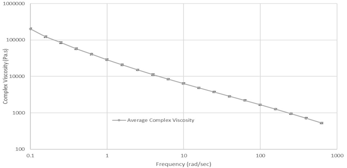
Figure 7. Average viscosity data from the viscosity data of 5 randomly loaded samples (20% CF ABS, 250°C, Air, 0.1% strain)
