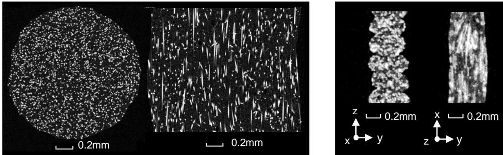
Fig. 4: Fiber orientation in the filament (left) and in the FDM part / strands (right)
