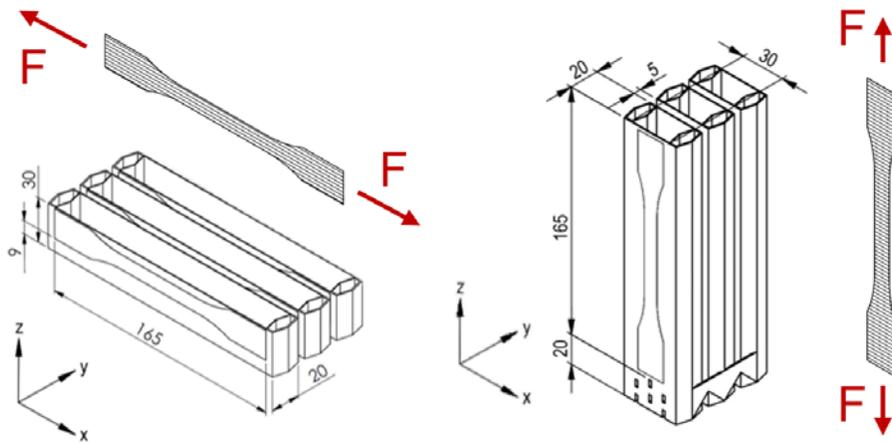
Fig. 1: Tensile bar in the x-direction (left) and z-direction (right)
