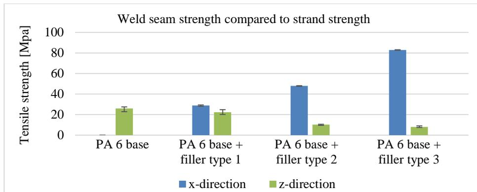
Fig. 3: Tensile tests (w/h-ratio = 2/1)
