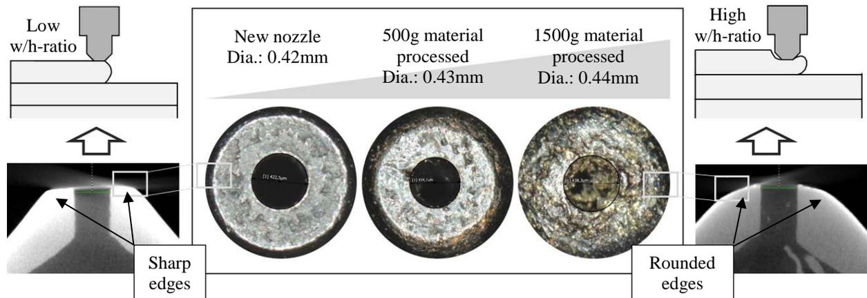
Fig. 7: Nozzle erosion for different w/h-ratios due to the processing of filled materials
