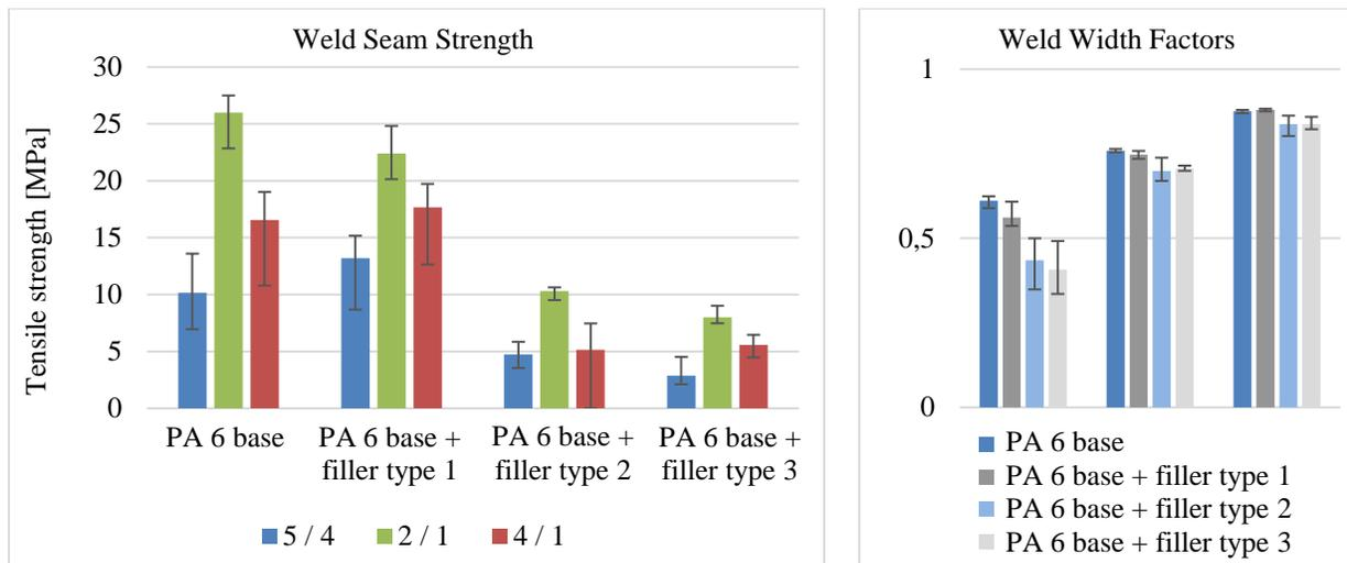
Fig. 6: Weld seam strength for different w/h-ratios
