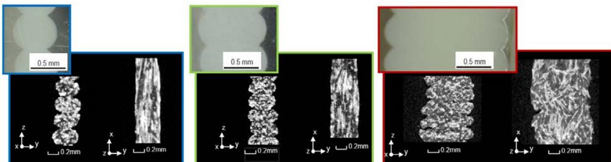
Fig. 5: Fiber orientation for different w/h-ratios (left: 5/4, middle 2/1, right: 4/1)
