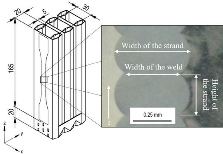
Fig. 2: Tensile bar in the z-direction
