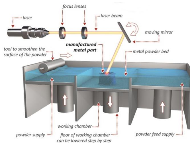
**Figure 2:** Schematic demonstration of the SLM process [6]
