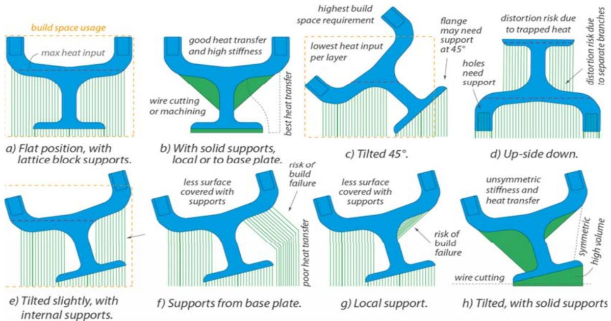
**Figure 13:** Different types of supports in various orientations of the same part leading to different manufacturability, laser scan area per layer, surface roughness, build height, etc. [30]
