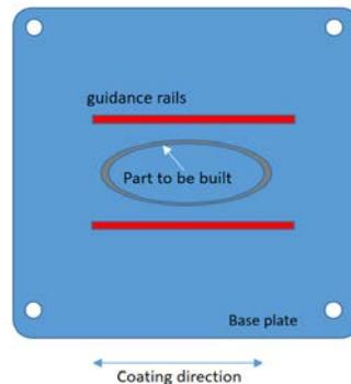
**Figure 11:** Rail type support structures to avoid tight contact between the part to be built and the coater leading to deformations and local dents (from top view of the base plate)
