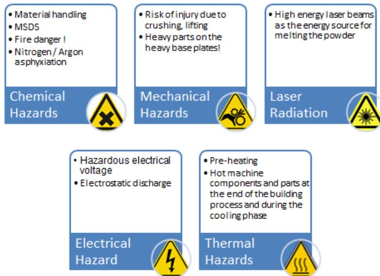
**Figure 5:** Different types of hazards related to the SLM process
