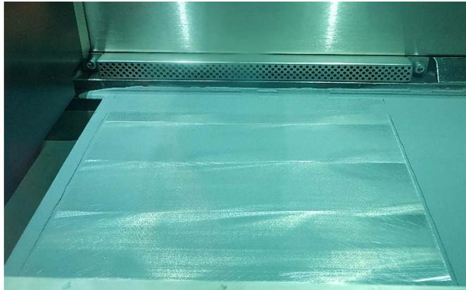
**Figure 7:** The very first layer of powder deposition on a DMLS machine ready to start a new job
