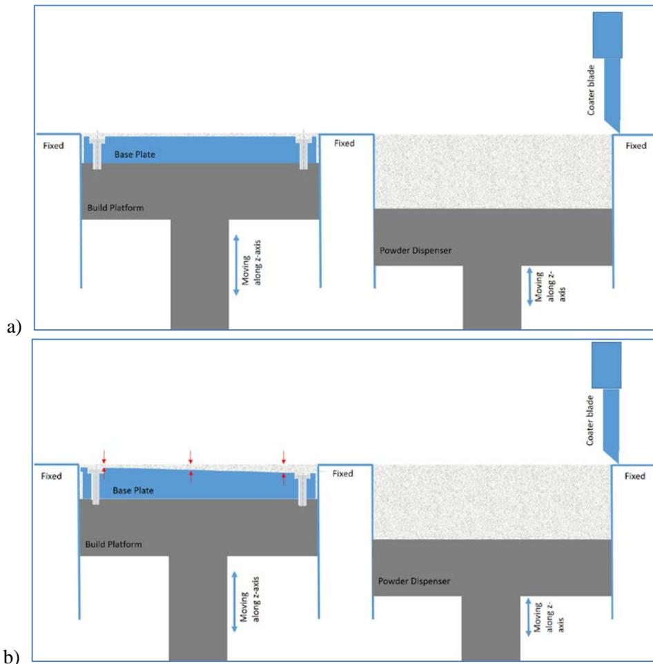
**Figure 8:** Inside the build chamber showing the main components (base plate, build platform, powder dispenser, coater blade) (not to scale) a) homogenous thickness of the first powder layer b) heterogeneous thickness of the first powder layer (see red arrows for the change of the thickness)
