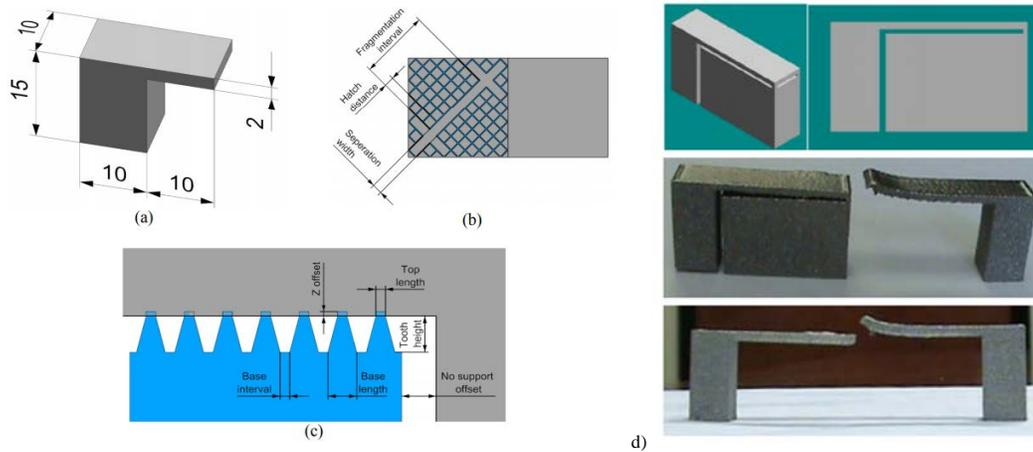
**Figure 10:** Designed part and dimensions for experiments (a), definitions for block supports (b), tooth dimensions (c) [25] contactless support structures and resulting geometries (d)
