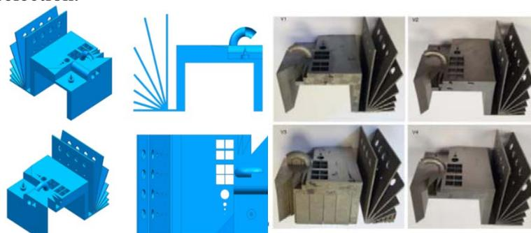
**Figure 3:** The benchmark design and obtained physical parts from 4 machine vendors presented in [6]
