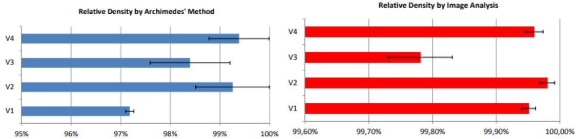
**Figure 4:** The specimen taken from the benchmark which was made by the Machine Vendor 1 (V1) presents very low Archimedes density compared to image analysis for the same specimen [6]
