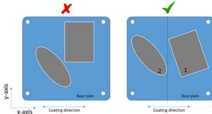
**Figure 12:** How to position the parts on the base plate a) a wrong positioning of 2 parts b) preferable positioning of the same parts
