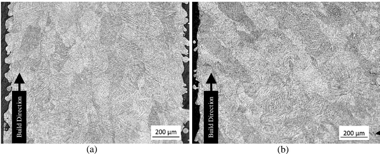
**Fig. 3.** Microstructure of L-PBF Ti-6Al-4V built in (a) vertical and (b) diagonal orientations.
