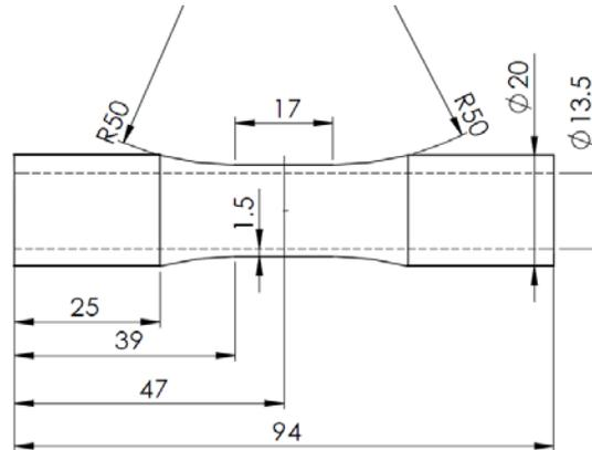
**Fig. 1.** Tubular multiaxial specimen with uniform gage section per ASTM standard E2207-15 [20]. All dimensions are in mm.
