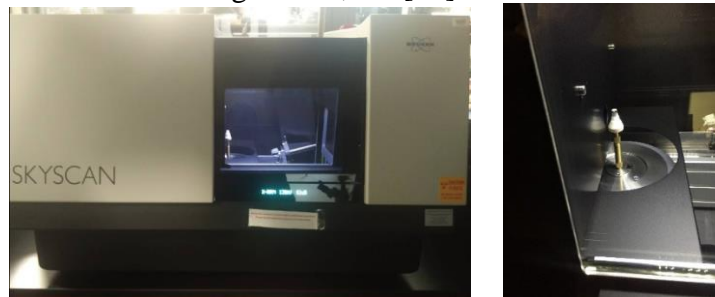
Figure 2: Specimen setup in the CT system (Left) and closed-up views (Right).
