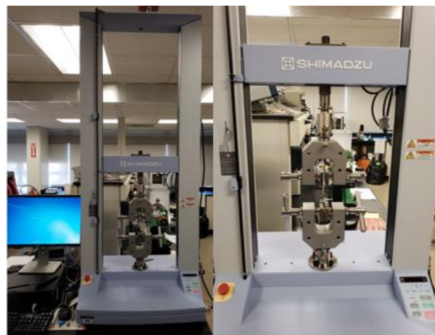
Figure 5. The AGS-X Universal Electromechanical Test Frame showing the mechanical grips.
