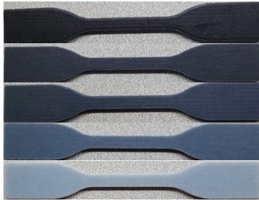
Figure 4. Fully printed specimens of different digital composites at 85\mu\text{m} voxel size.
