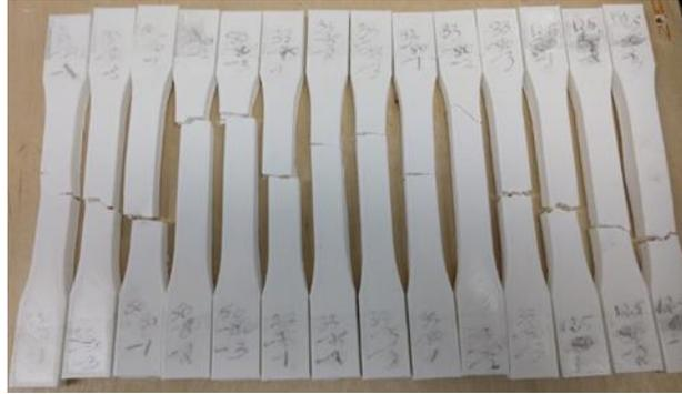
Figure 8:- Fractured set of specimens after mechanical testing
