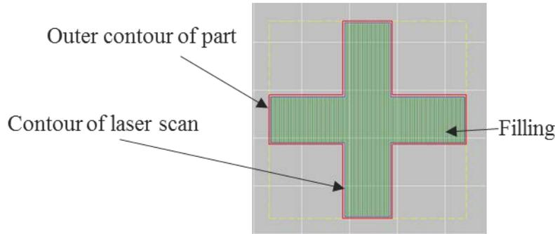
Figure 1: Laser scanning lines of the build part filling (green) and contour (red)
