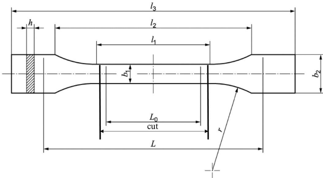
Figure 2: Cut-out of tensile specimen (DIN EN ISO 527 1A) for XCT-scans
