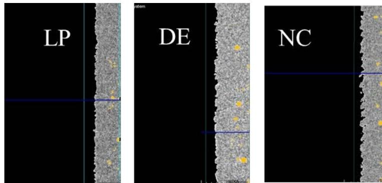
Figure 4: XCT-Scan sections of specimens LP, DE and NC to regard the surfaces
