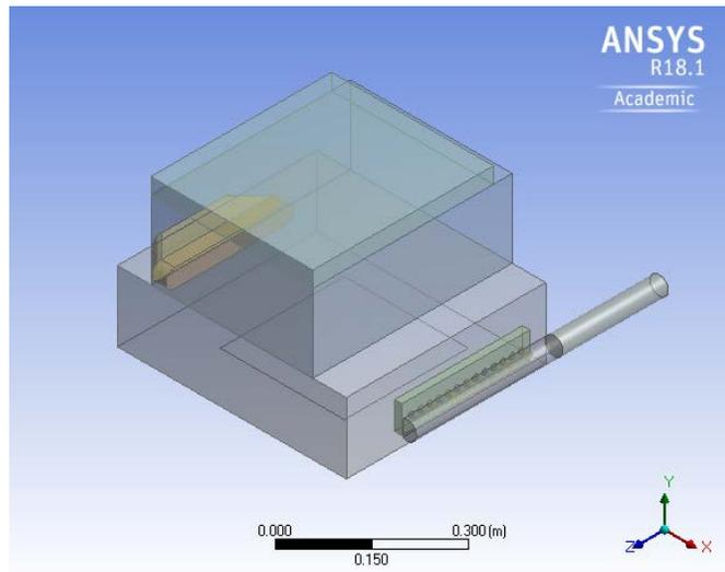
Figure 1, Sketch of the RENISHAW AM250 chamber
