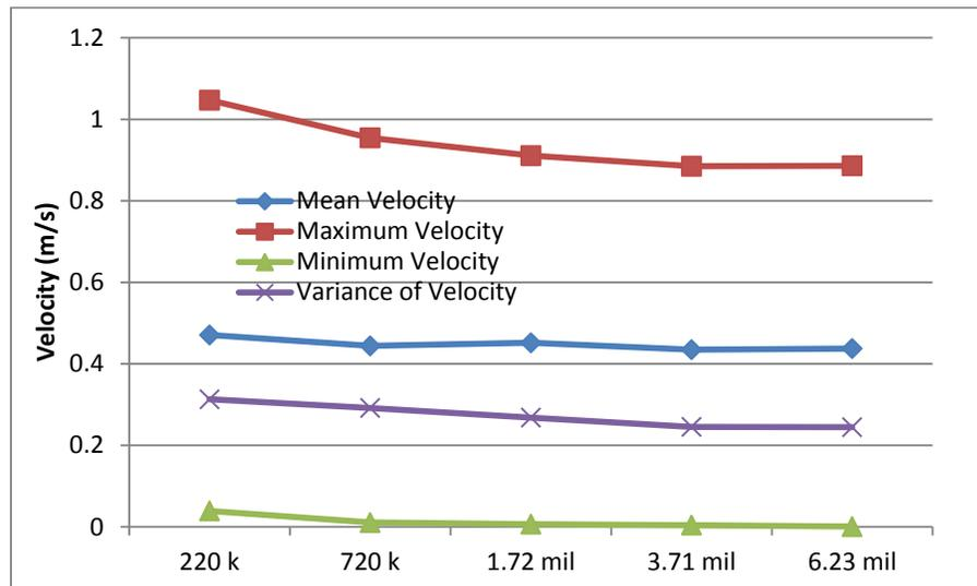
Figure 2, Grid independence study for velocity
