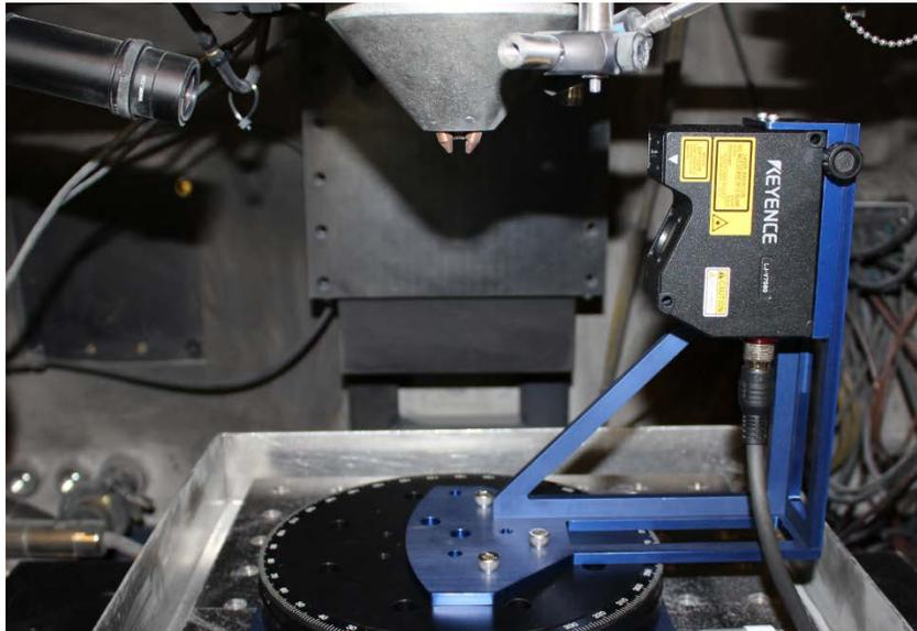
Figure 8: 2D OEM Laser Profiler
