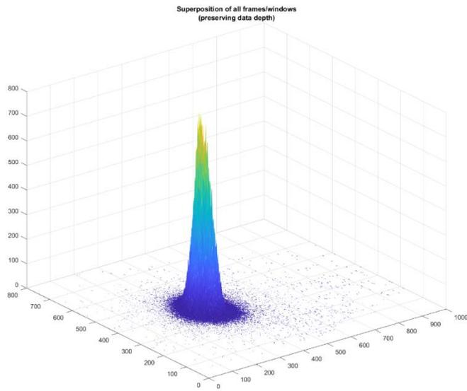
Figure 12: Superposed data frames from 2D OEM Laser Profiler showing average flow profile over 80 s duration
