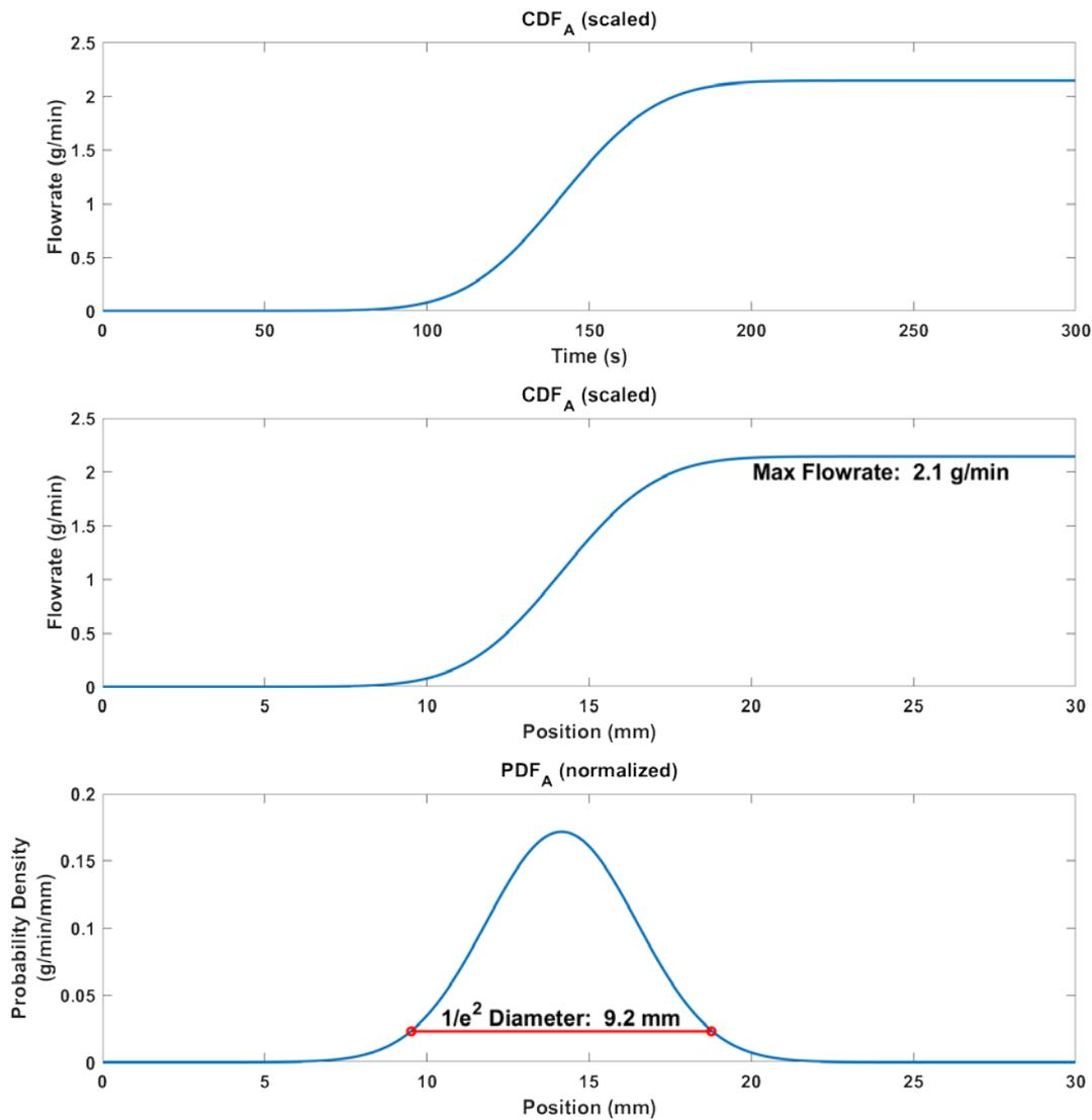
Figure 11: Idealized (i.e., no oscillation), curve-fitted portion of 1D Knife-edge Profiler data
