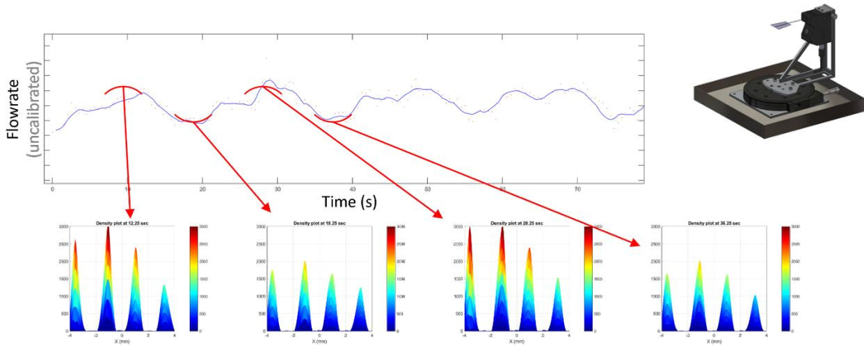
Figure 14: 2D OEM Laser Profiler data collected at exit of powder nozzles
