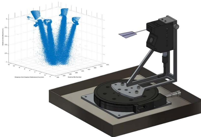
Figure 5: 2D OEM Laser Profiler with representative dataset
