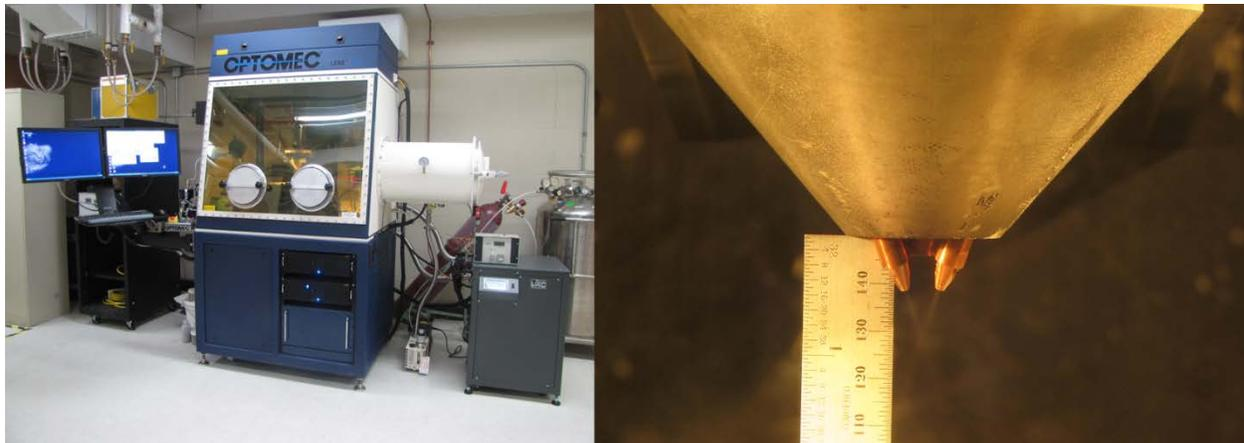
Figure 6: Optomec LENS MR7 DED system (left) and powder nozzles (right)
