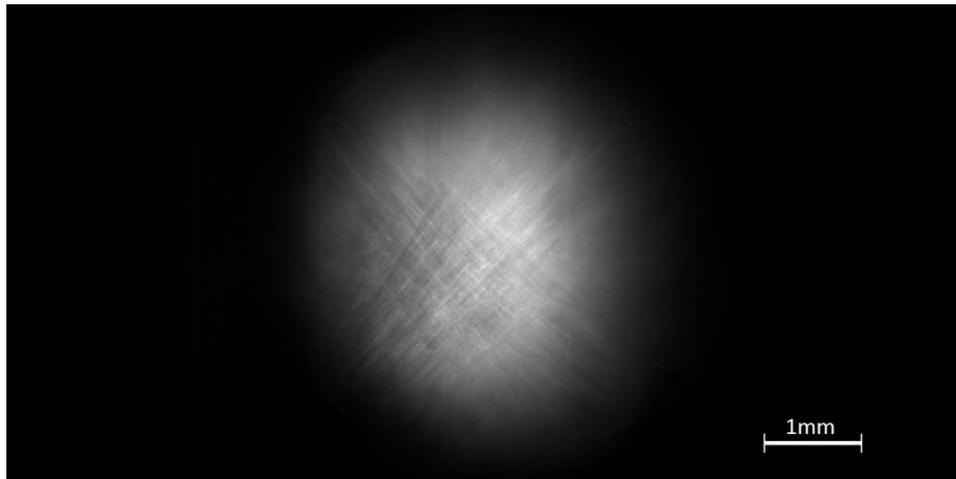
Figure 3: 2D Laser Line Scanning image of coalesced powder from four nozzles
