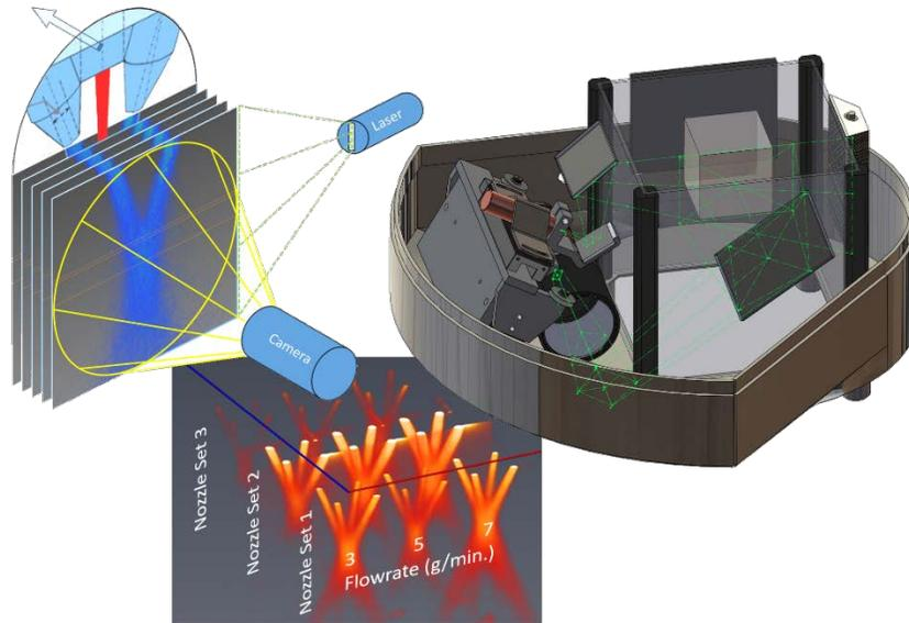
Figure 2: 3D Custom Laser Profiler method and representative datasets
