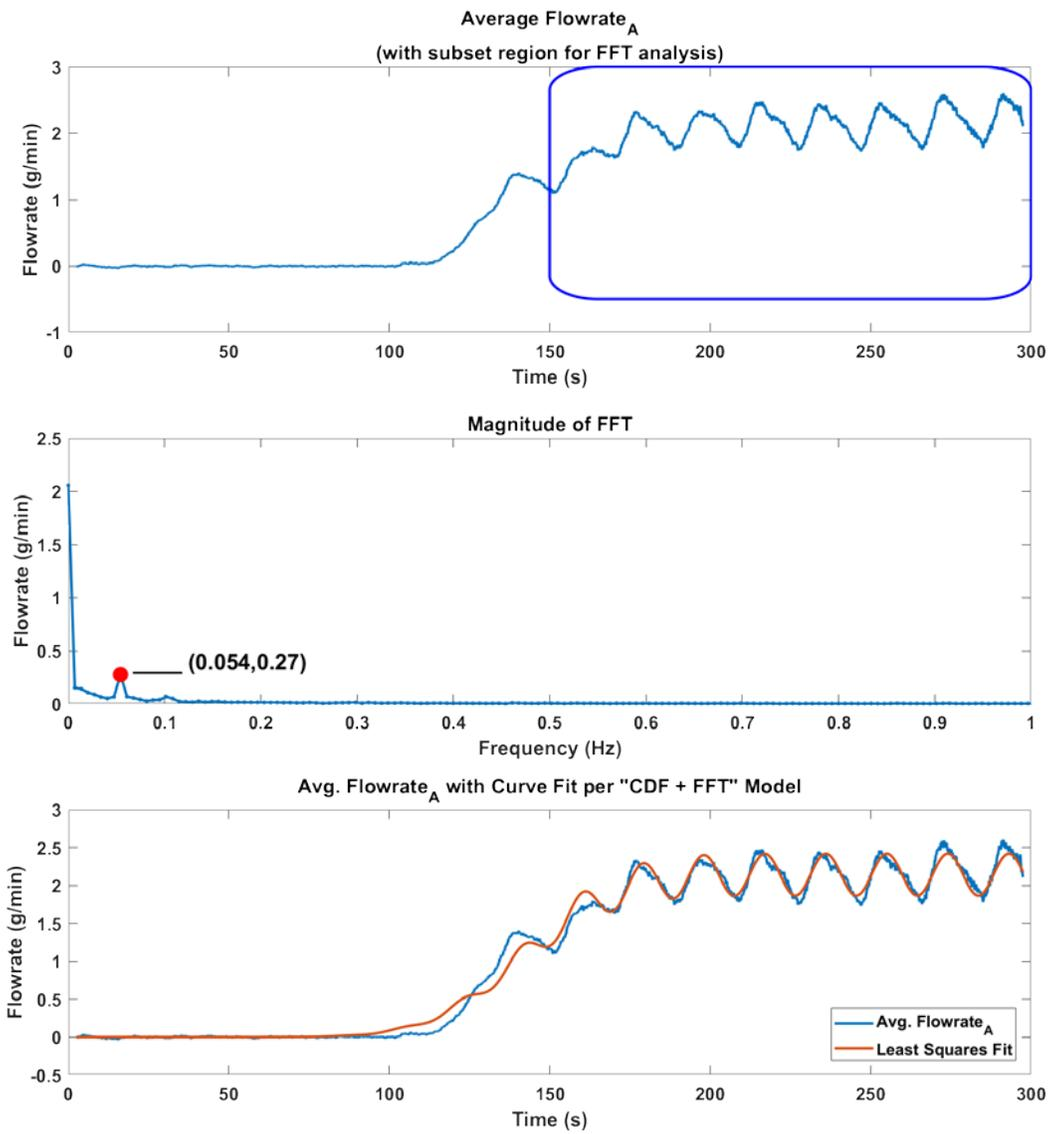
Figure 10: 1D Knife-edge Profiler data with CDF + FFT curve fit
