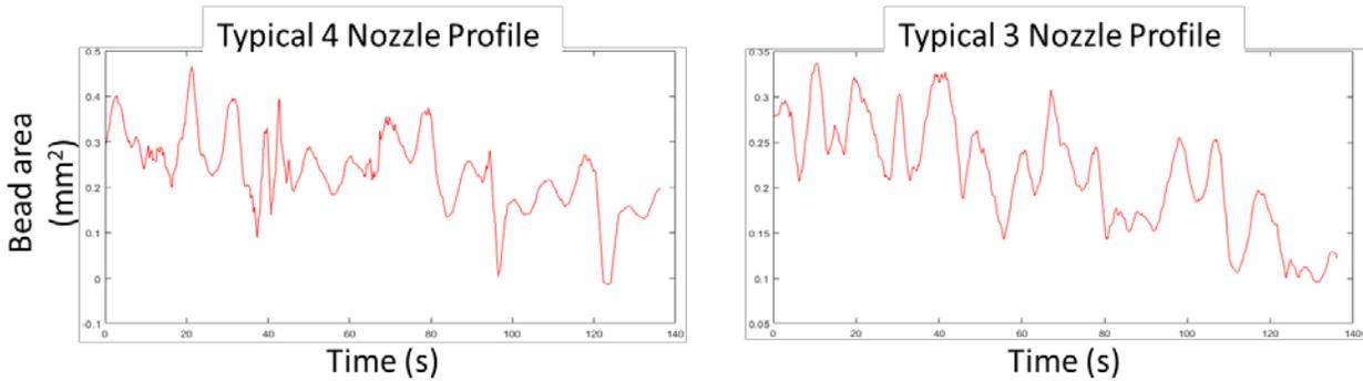
Figure 16: Variation in deposition bead area over time
