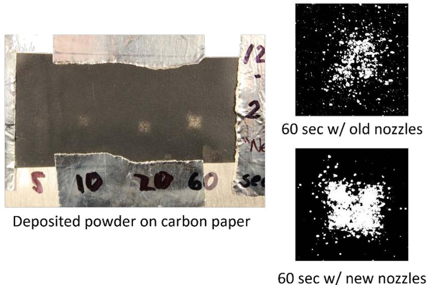
Figure 1: 2D Carbon paper impressions/datasets
