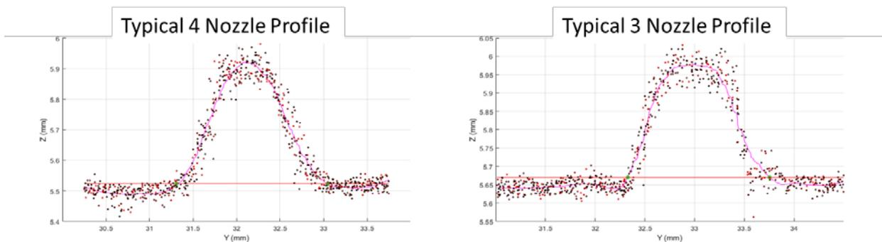
Figure 15: Typical deposition profiles using 4 (standard) or 3 (one quadrant plugged) nozzles
