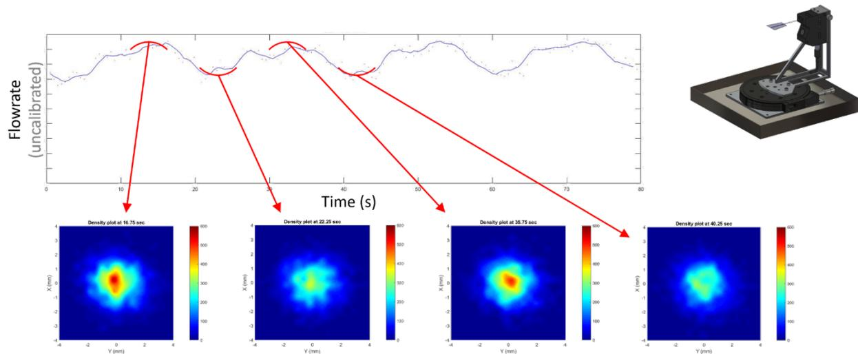
Figure 13: 2D OEM Laser Profiler data collected at convergence point of powder streams
