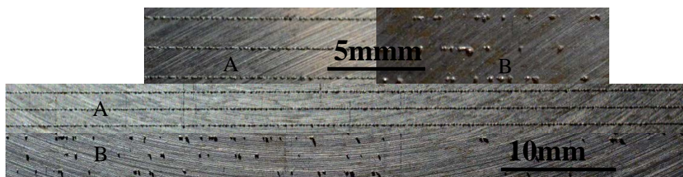
Figure 2: Maraging steel tracks on the substrate at 305 W laser power and scanning speed of 1.1m/s at 50 \mu\text{m} powder layer thickness (Optimal; A) and 300 \mu\text{m} (non-optimal; B)
