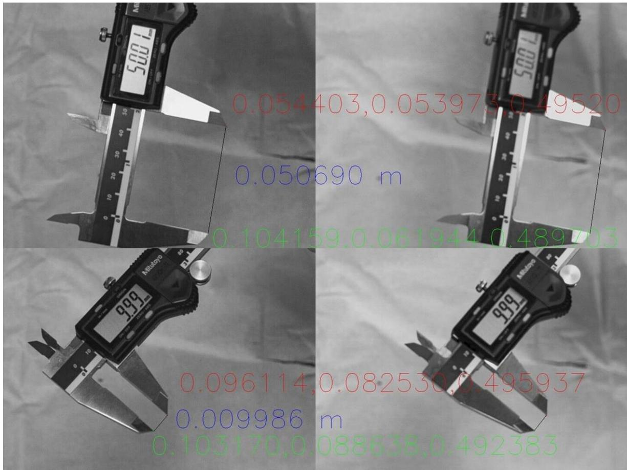
**Figure 3** - Stereovision quality assurance using a caliper (50.01 mm top, 9.99 mm bottom).
