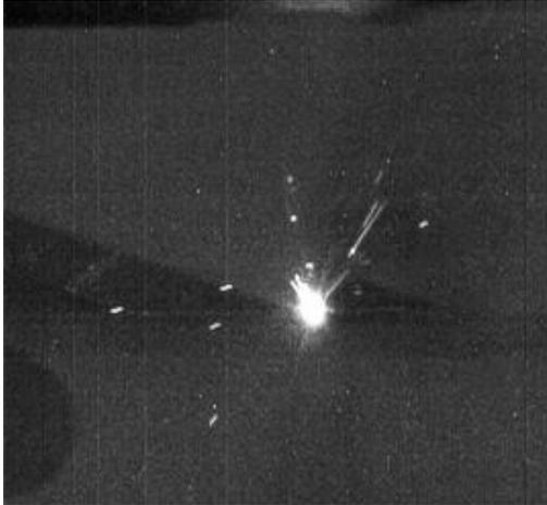
**Figure 6** - Spatter calving where new spatter particles have been formed and are being ejected.
