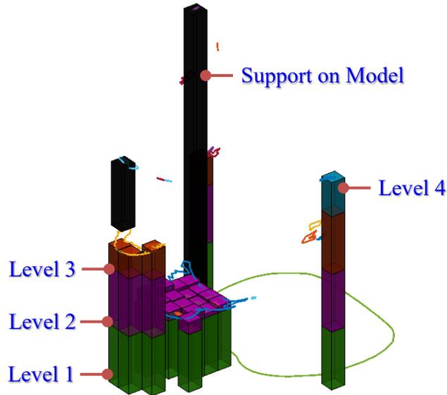
**Figure 3.** Conventional support structures split into levels with the given modular block height for the Atatürk model. The boundaries show the areas which require support.
