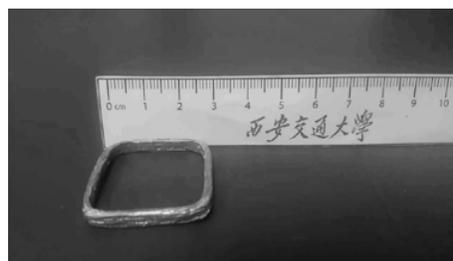
FIG. 4 The frame printed by FTP.
