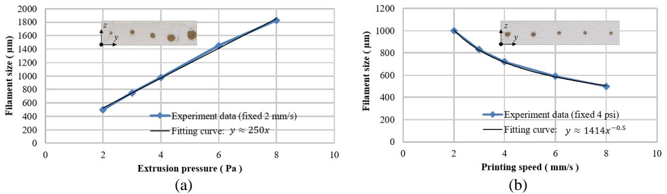
Figure 2. Effects of (a) extrusion pressure and (b) printing speed on extruded filament size.
