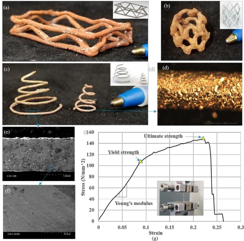
Figure 3. Test cases: (a) a lattice structure, (b) stent structure, (c) cone springs, (d) optical microscope image of springs, (e) and (f) SEM images of printed samples, (g) tensile test of a fabricated specimen.
