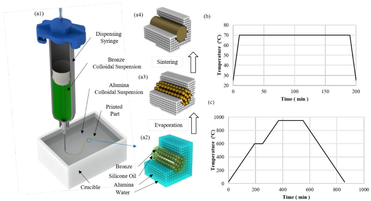
Figure 1. (a) Schematic diagram of II-DMD; (b) temperature schedule for drying; (c) temperature schedule for sintering.
