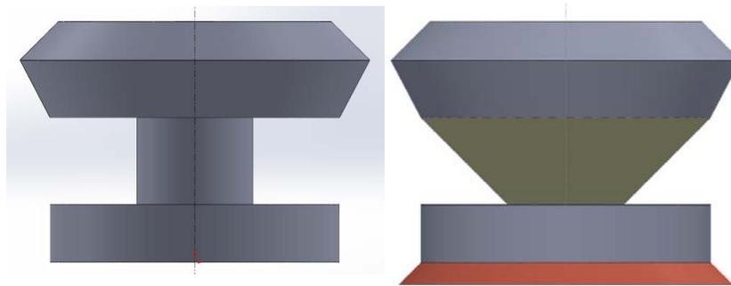
Figure 5 – Front view of the finished part example (left) and part with supports and sacrificial material (right).
