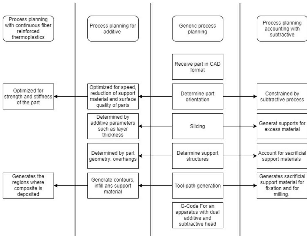
Figure 3 – Generic process planning and different adaptations for additive, subtractive and reinforced additive.
