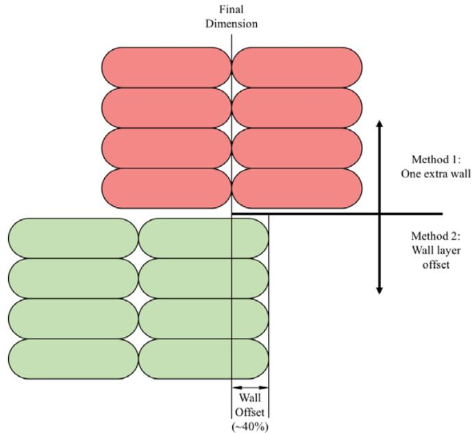
Figure 2 – Two possible methods for machining excess material
