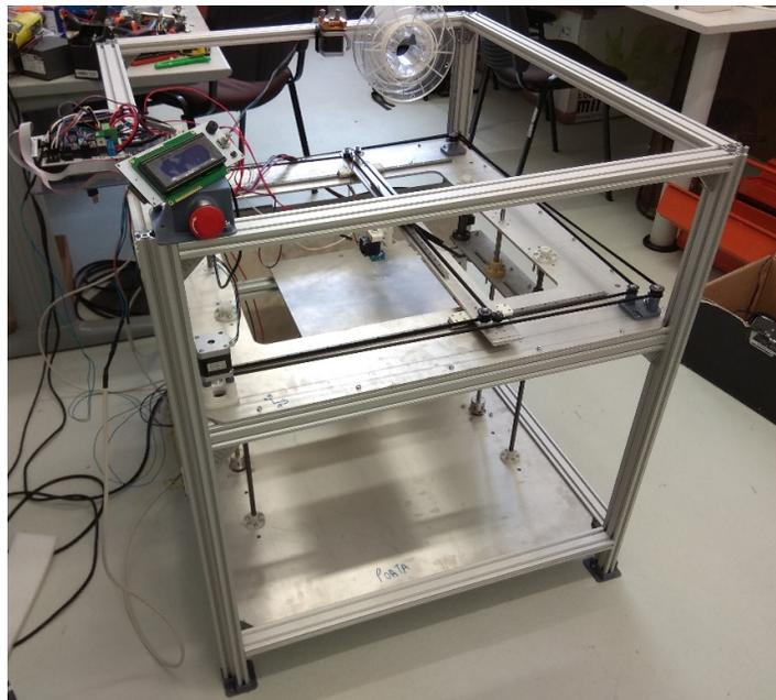
Figure 4 – Experimental rig for hybrid additive and subtractive processes
