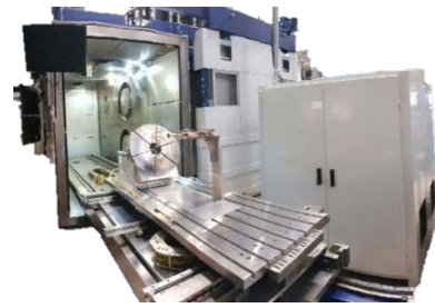
Figure 12 UBC EB 150 kV machine
