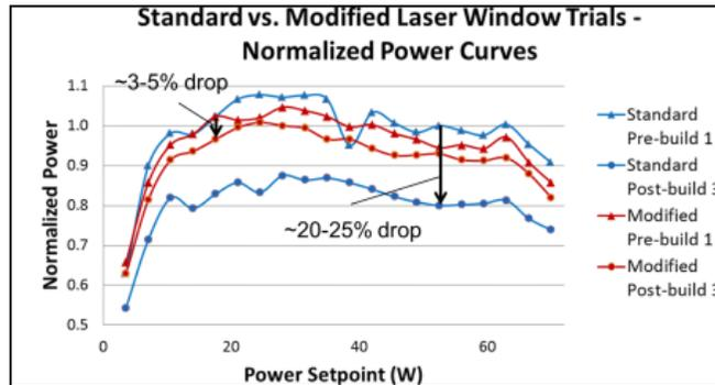
**Figure 3: Laser power attenuation for standard and modified laser window [8]**
