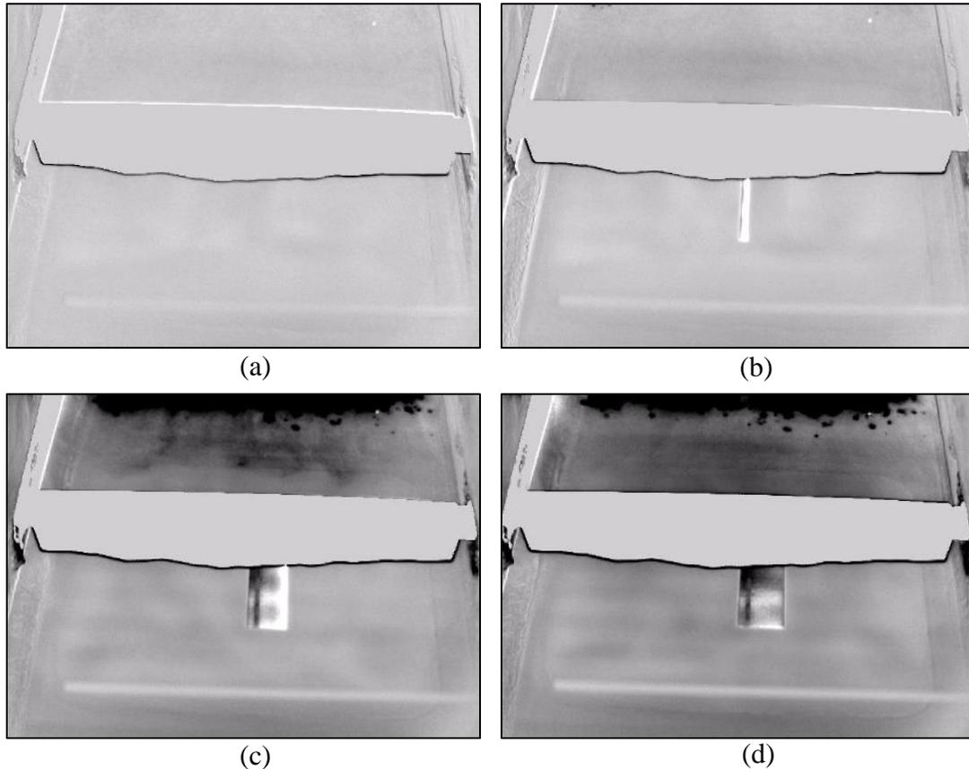
**Figure 11: Thermal images of a pre-sintered powder bed (a), powder bed during sintering (b), powder drop from storage hopper (c), continued turbulence after powder drop (d)**
