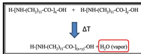
**Figure 2: Post-condensation reaction between two polyamide monomers [5]**
