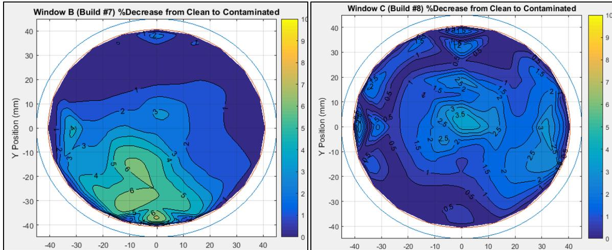
**Figure 10: Contour plots of % change in attenuation from clean to contaminated windows**
