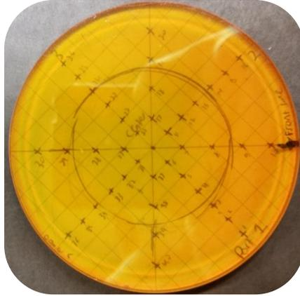
**Figure 7: Zinc selenide laser window overlaid on measurement grid**
