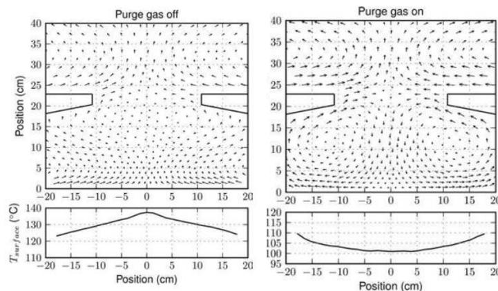
**Figure 4: Steady-state convection, warm-up after 1600sec, vectors of gas velocity at mesh nodes. Lower axes show powder bed surface temperature, initial temp 60C [9]**
