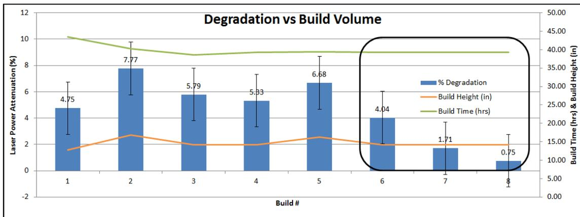
**Figure 8: Correlation between laser power attenuation and build parameters**
