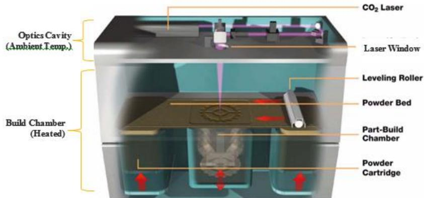
**Figure 1: Schematic of 3D Systems Sinterstation SLS Machine [4]**
