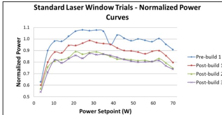
**Figure 5: Measured laser power before and after 3 builds in Sinterstation 2500 at SDM; builds 1 & 2: 16” high, build 3: 6” high [5]**
