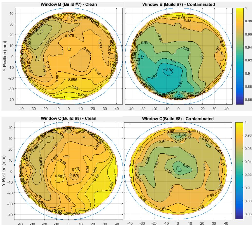
**Figure 9: Contour plots of laser power attenuation due to contamination for builds 7 & 8**
