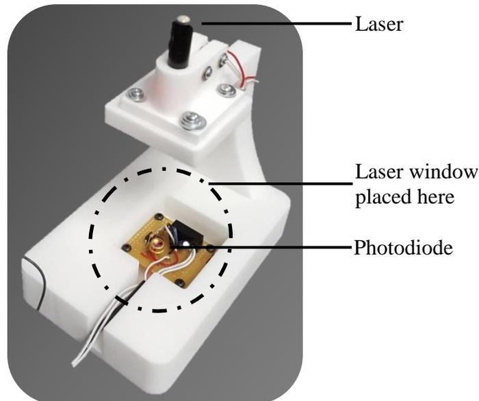
**Figure 6: Low cost laser/photodiode power meter**
