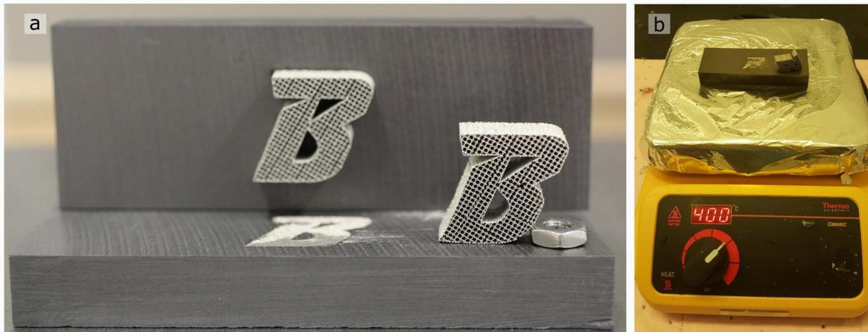
Figure 3: a) Stainless steel logo printed on graphite. b) Removing printed part using hot plate.
