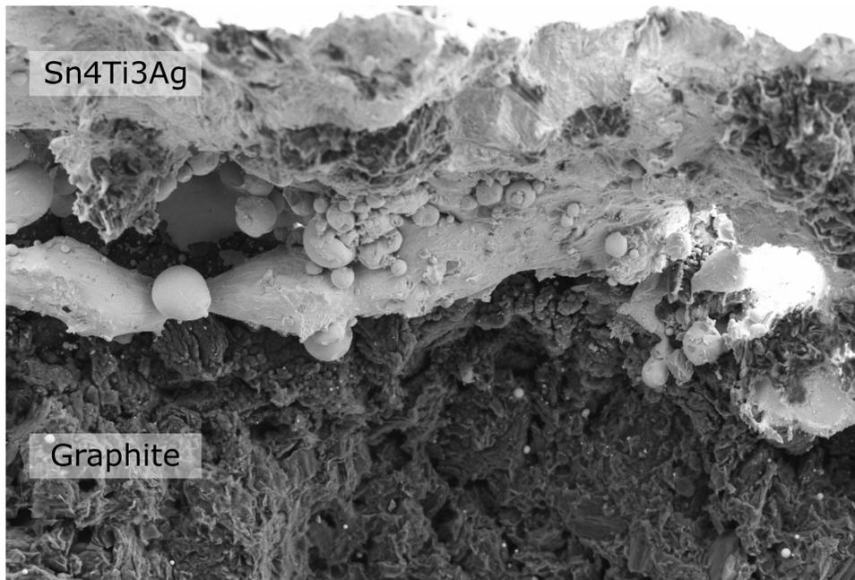
Figure 8: Unpolished scanning electron microscopy of graphite -Sn4Ti3Ag interface (EHT= 15kV, WD=9.9 mm, SE2 detector).
