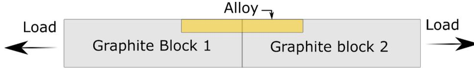
Figure 5: Schematic of the shear lap test
