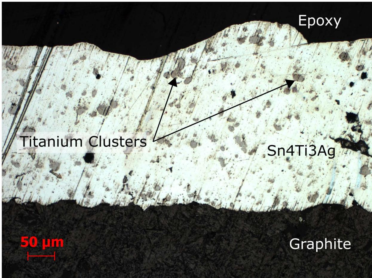
Figure 7: Optical image of the interface containing titanium-tin intermetallic phases.
