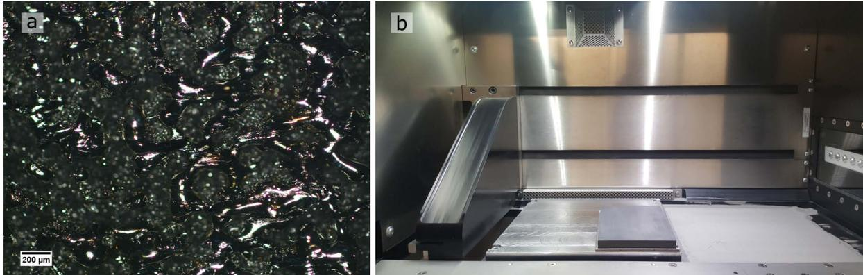
Figure 2: a) Optical image of stainless steel 316L deposited on graphite. b) Fixture designed to hold graphite substrate on build platform of EOS M290.
