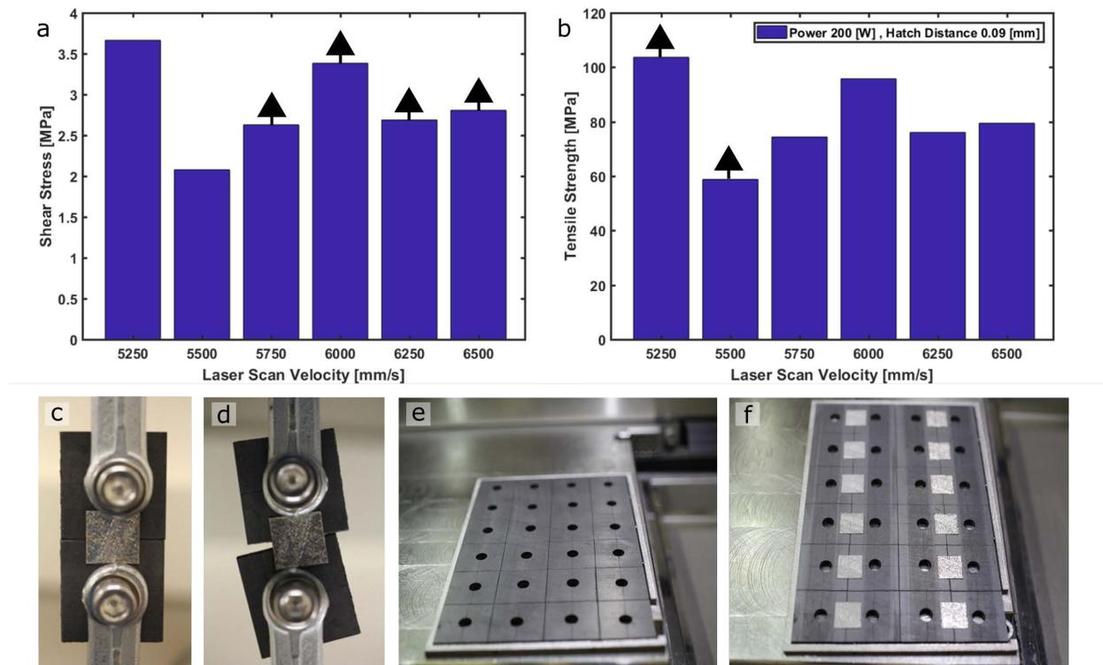
Figure 6: Interfacial strength of the graphite-metal bonding at various laser scan velocities (a, b). Sample preparation for tensile test (c, d, e, f).
