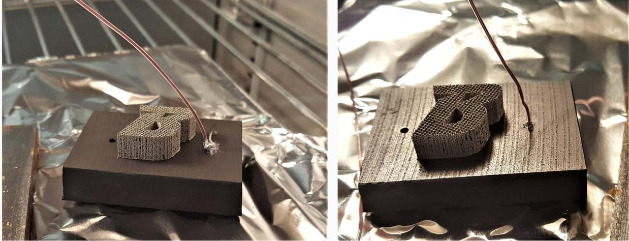
Figure 10 Two stainless steel parts after thermal cycling test
