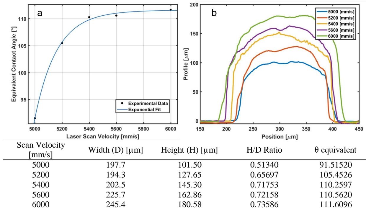
Figure 4: a) Contact angle versus laser exposure parameters, b) profilometry scans used to determine contact angle
