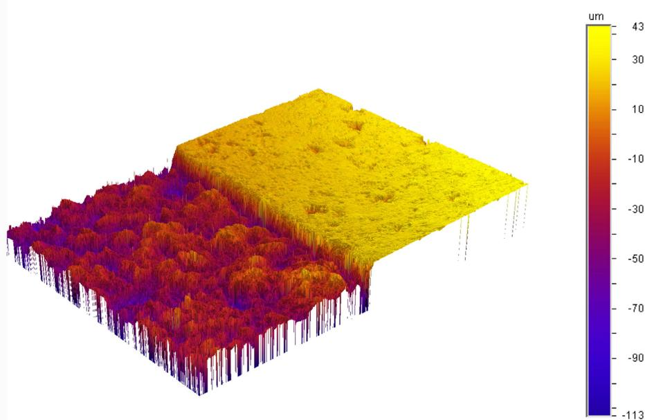
Figure 1: Optical profilometry of ablated graphite. The area scan size is  $1.7 \times 2.3$  mm.
