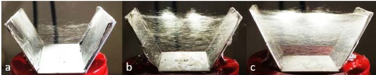
Figure 3. Formation of the 3D nanofiber scaffold. (a)-(c) represent 10 secs, 30 secs, and 60 secs after electrospinning, respectively.
