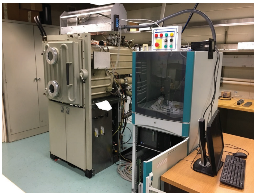
Figure 12. Rensselaer's research SLM system. The mechanical components are housed in the repurposed vacuum vessel to the left. The controller is housed in the cabinet to the right.
