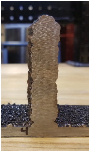
Figure 6: Four bead wall cross section.
