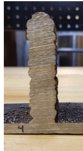
Figure 7: Second four bead wall cross section.
