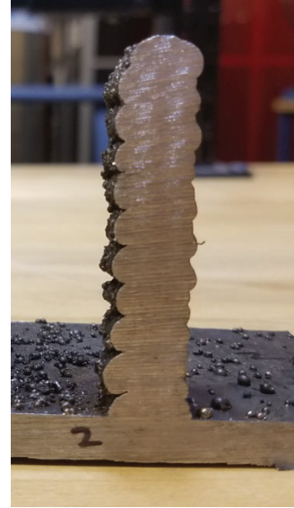
Figure 5: Cross section near end showing additional material flow.
