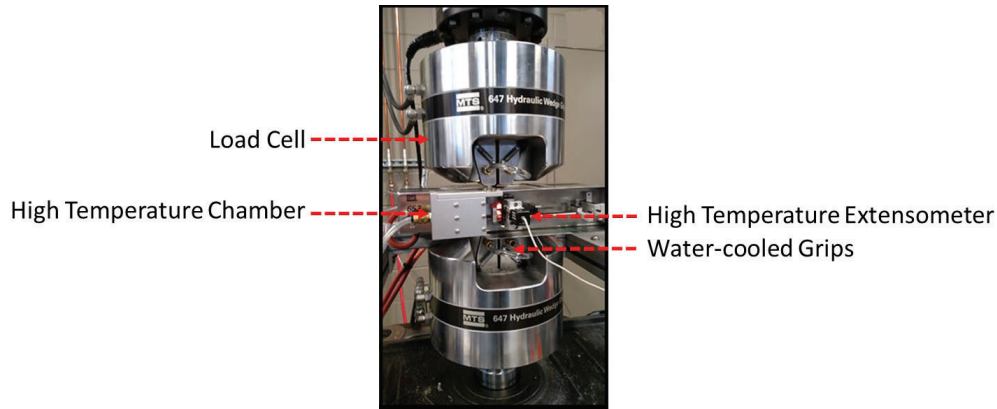
Figure 2. High temperature fatigue test setup showing all of equipment used in the study.
