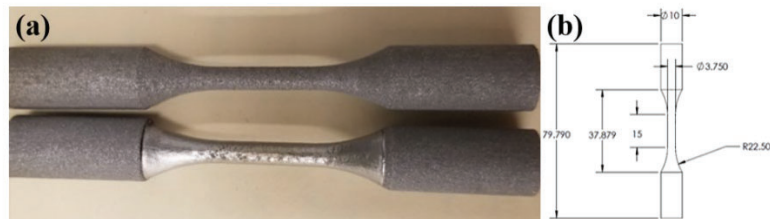
Figure 1. (a) Optical images of parts before (top) and after (bottom) the laser surface treatment. (b) Dimensions of the fabricated parts.
