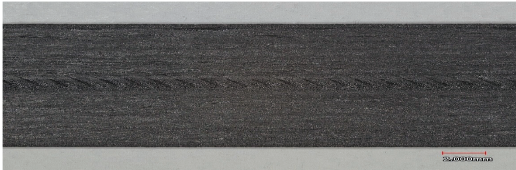
Figure 7. Cross section of a paused print showing the fiber region and onyx region
