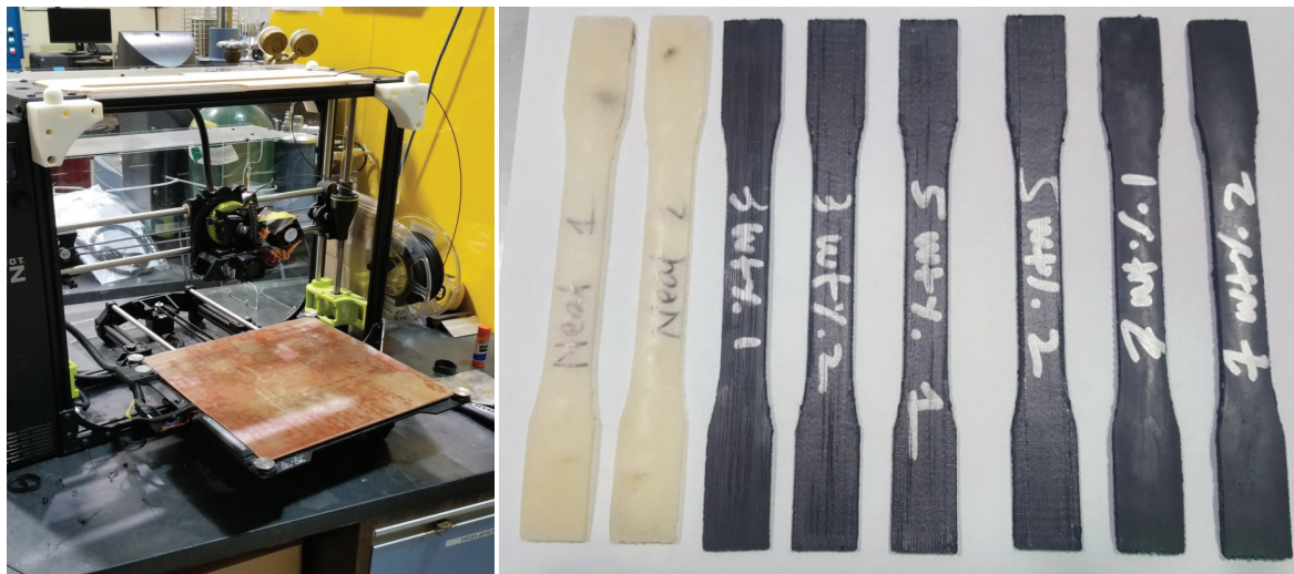
Figure 1. Lulzbot TAZ 6 Printer and Printed Tensile Samples
