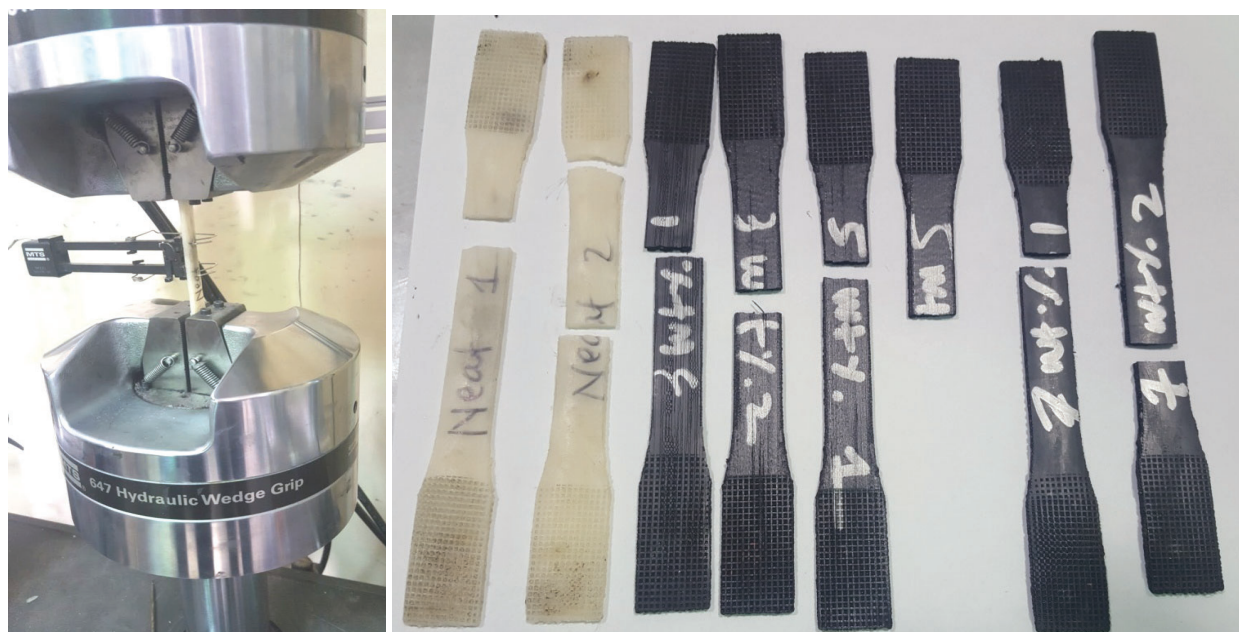
Figure 2. Tensile Testing Setup and Tested Specimens.
