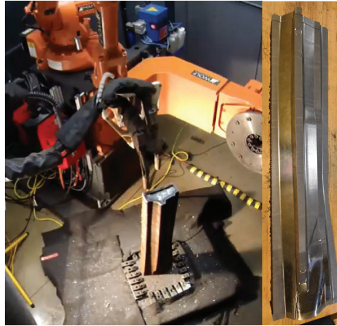
Figure 9. Printing a press using stainless steel and mild steel. Left) Die while being printed. Right) Die after machining
