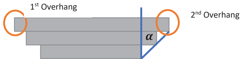
Figure 1: Schematic showing 1 st and 2 nd overhangs in subsequent layer scans during fabrication of a single-track, thin wall with negative draft angle
