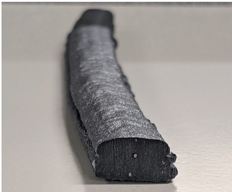
Figure 5: Cross Section of beads with wire
