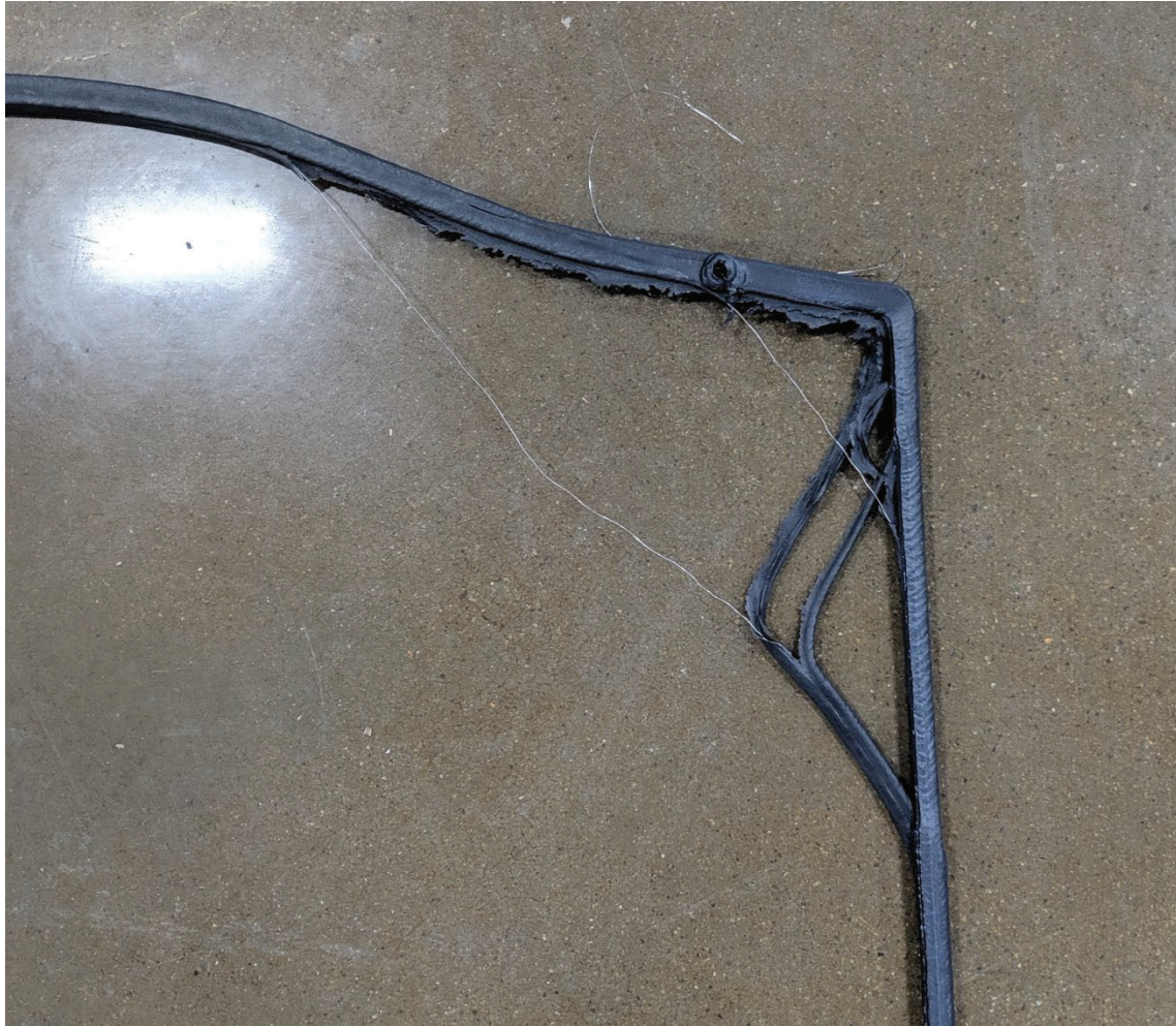
Figure 3: Failed part from motor running too slowly
