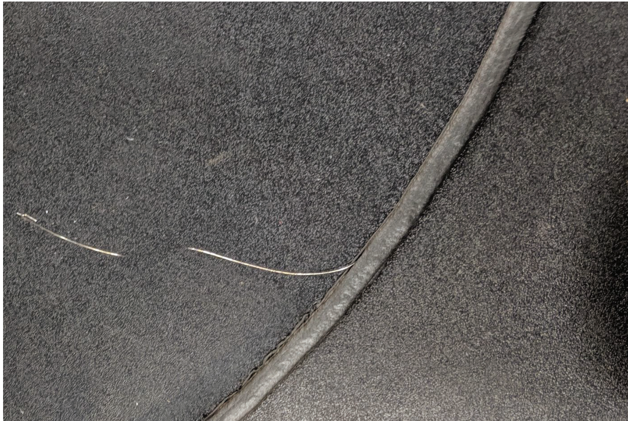
Figure 7: Wire lead out on bead printed without tamper
