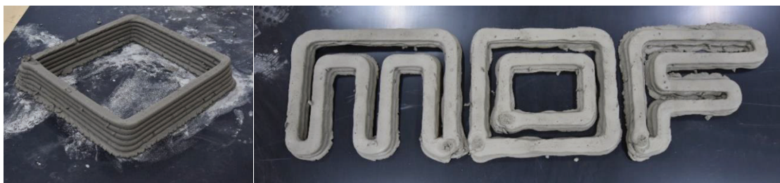
Figure 13. Concrete bead calibration square (left) and ‘MDF’ printed out of concrete using the SkyBAAM system (right)
