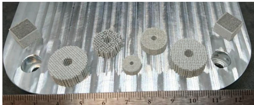
Fig. 4. Cubes printed with hatch and border speed of 400 m/s and 150 mm/s, respectively. First attempt of printing lattices are also shown
