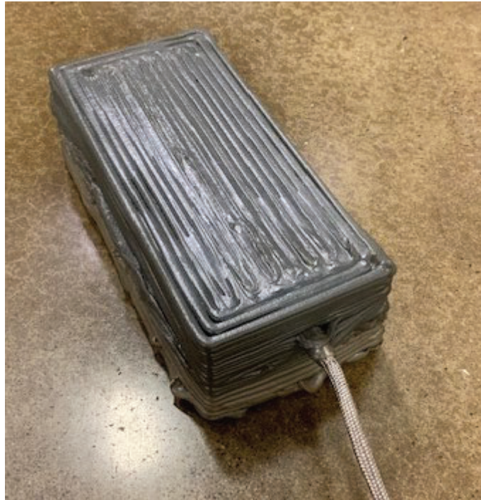
Figure 10: Finished printed part with heater cartridge successfully placed in the center of the part
