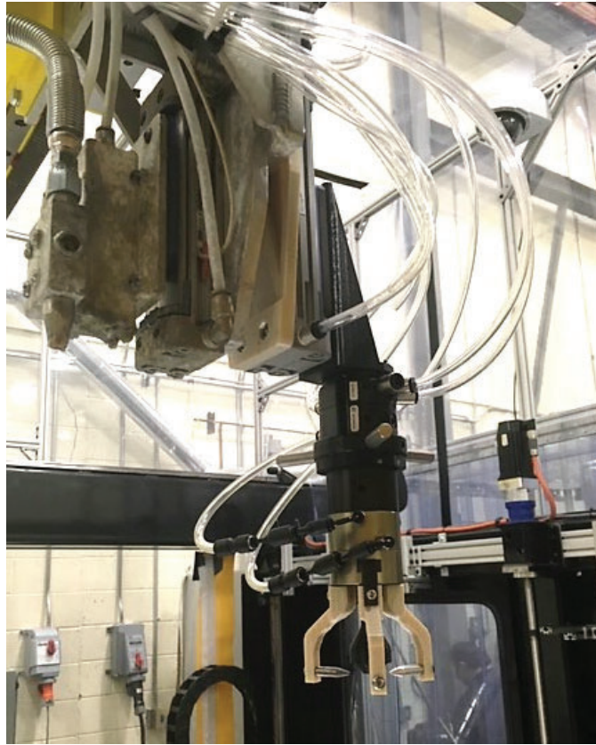
Figure 14: Full tool changer assembly demonstrated on MVP's thermoset printer
