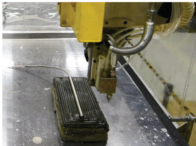
Figure 9: The heater cartridge successfully placed in the middle of the part mid-print
