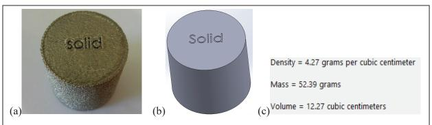
Figure 2 - (a) Solid cylinder build to calculate the density of Ti-6Al-4V after EPBF, (b) CAD model of the cylinder, and (c) the mass properties results from SolidWorks 2018.
