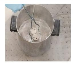
Figure 4 – (Left) Parts before they are submerged inside a pot with liquid nitrogen. (Right) Parts submerged inside a pot with liquid nitrogen.
