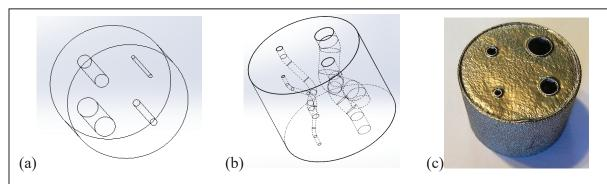
Figure 1 – (a) CAD cylinder design with straight channel features, (b) CAD cylinder design with curved channel features, and (c) Additive Manufactured Cylinder.
