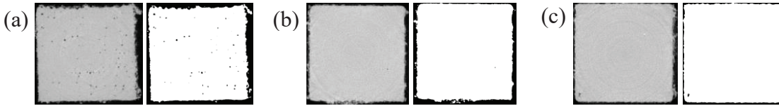
Fig. 8. Example of one image slice and its corresponding binary image for (a) high (b) medium and (c) low energy cases
