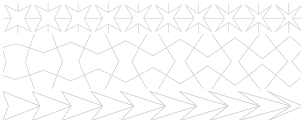
Figure 2: Linear gradation of the three patterns (from top: star, bow, and arrow), open on the left to closed on the right. As the pattern becomes more closed and the internal angles more acute the magnitude of the Poisson's ratio increases.
