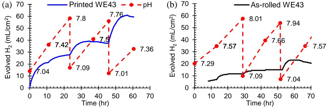
Fig. 9 H<sub>2</sub> evolution in concentrated NaHCO<sub>3</sub> solution for (a) printed and (b) as-rolled WE43.
