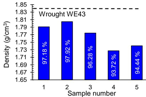
Fig. 7 Dependency of the density of printed WE43 corrosion samples on their position in the print chamber. Percentage values represent relative density compared to as-rolled WE43.
