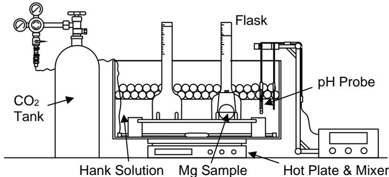
Fig. 8 Experimental setup for corrosion testing.
