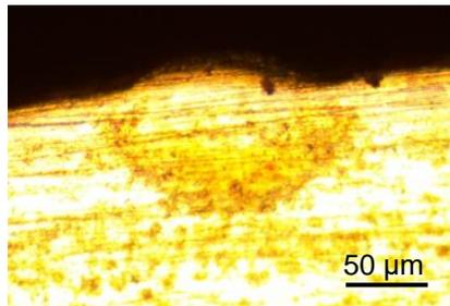
Fig. 2 Melt pool obtained at 135 W laser power and 700 mm/s scan speed.
