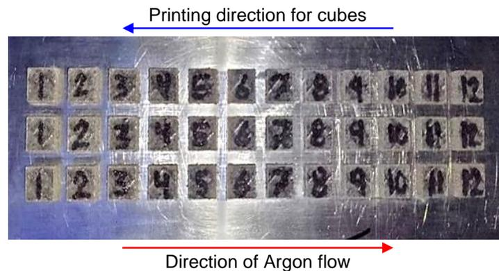
**Fig. 3** Cubes for density measurements printed on a baseplate.
