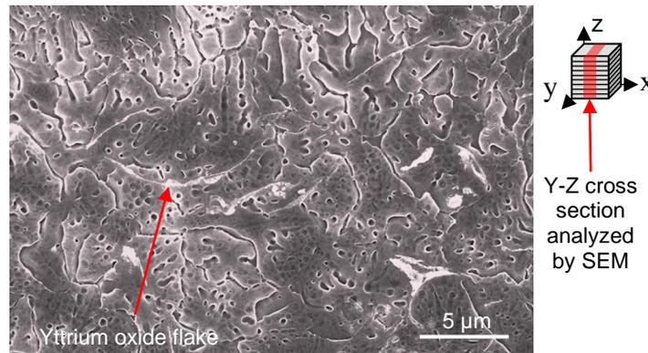
**Fig. 4** Microstructure of WE43 printed with laser power of 135 W, scan speed of 700 mm/s, and hatch spacing of 0.12 mm.
