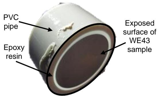
Fig. 5 WE43 sample for corrosion testing.
