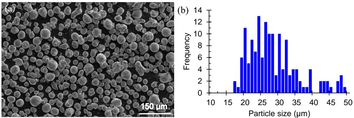
Fig. 1 WE43 powder (a) morphology and (b) particle size distribution.
