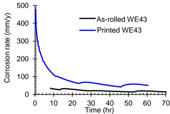
Fig. 10 Corrosion rates of printed and as-rolled WE43 in concentrated NaHCO<sub>3</sub> solution.
