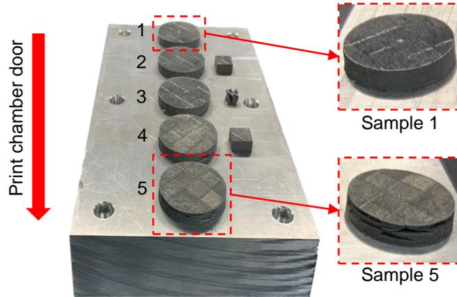
Fig. 6 Printed WE43 corrosion test samples. Samples 1-3 showed no delamination while samples 4 and 5 delaminated.
